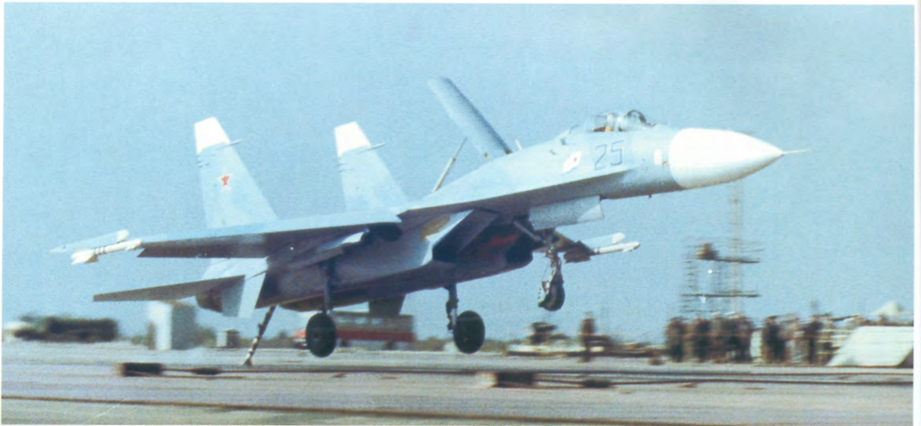
Before actually landing aboard a ship, a lot of ski-jump assisted take-offs and arrested landings were performed at Test Center in Crimea. The Soviet Navy flag near the number "25" identifies this aircraft as one designated for naval service. Note dorsal airbrake. (Sukhoi Design Bureau)
