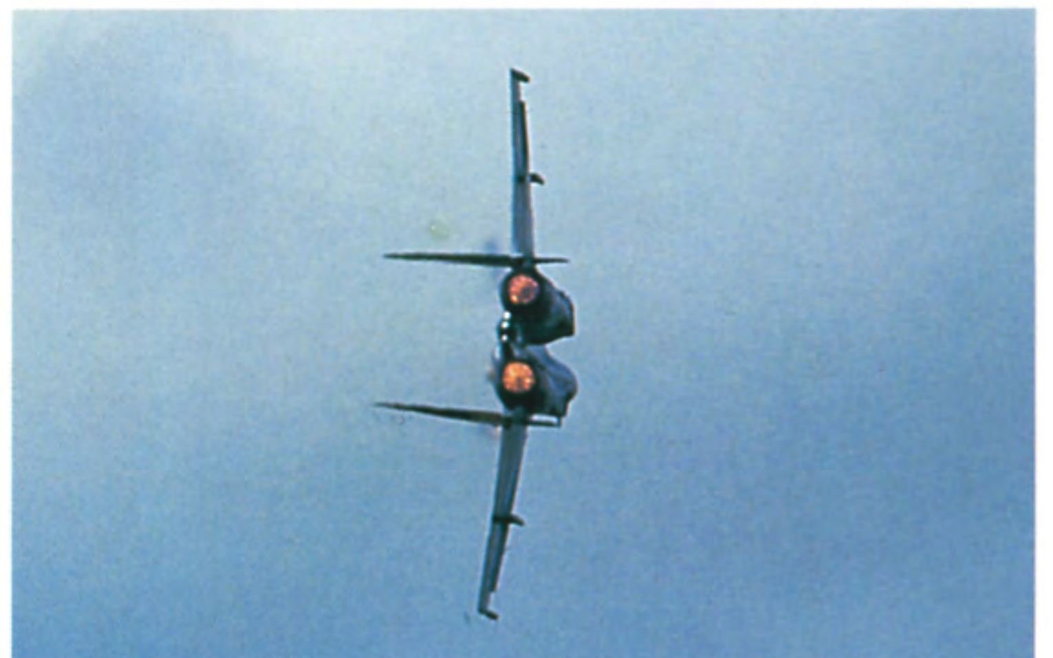
Rear in-flight view of the Su-27 flying with afterburner lit. Visible convergent/divergent nozzles are the radial fuel sprays in the A/B flame stabilizers. The aircraft is powered by two Lyulka AL-31F engines. (Sergey Pashkovsky)
