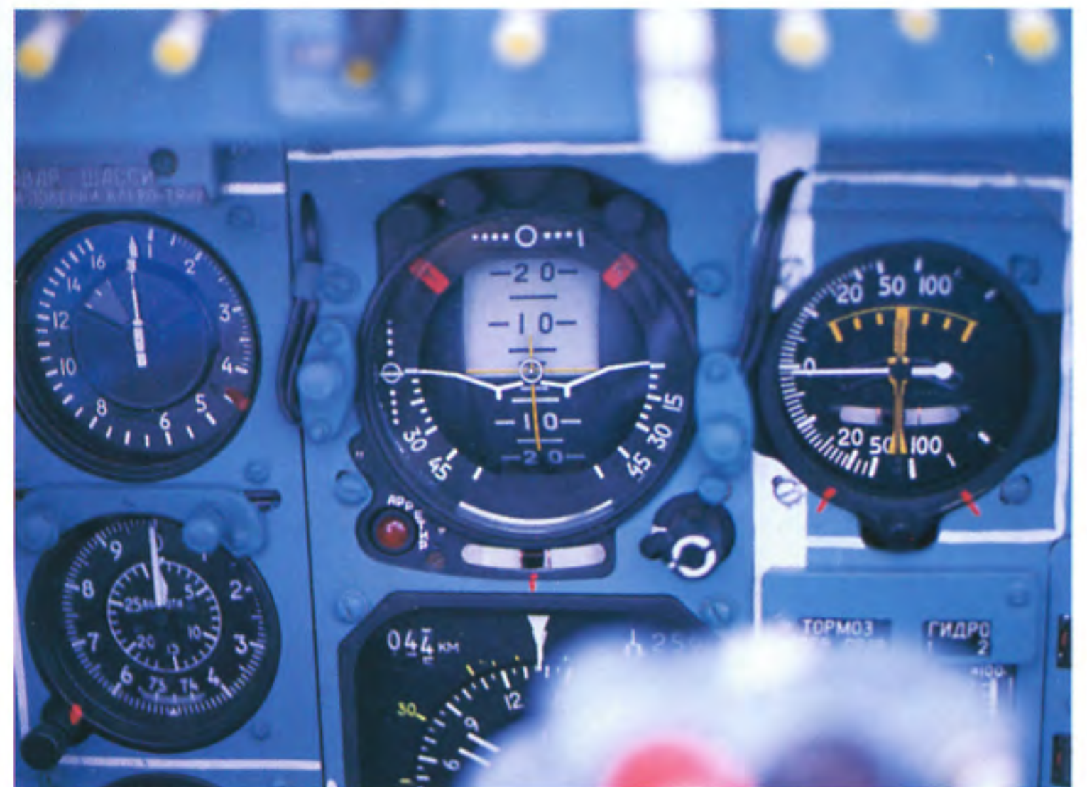
Central instrument panel deals with the main instruments, indicated airspeed indicator, barometric altimeter, attitude directional indicator (ADI) and turn and slip indicator.
