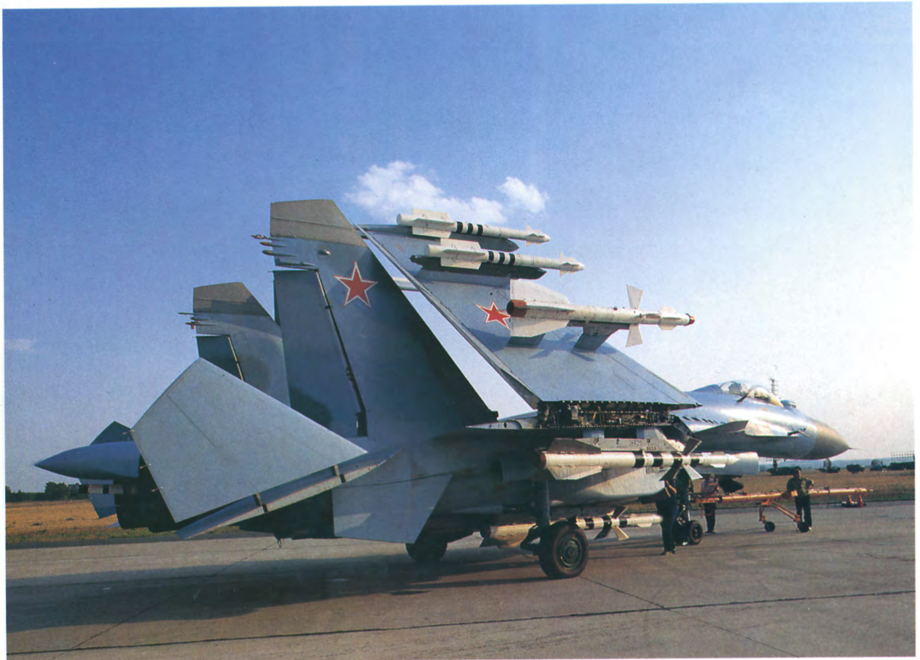
In order to save parking space on the deck of the carrier and provide adequate hangar stowage, certain modifications are made to carrier-based aircraft. Two of these are shown here: folding wing and folding stabilizer. The central tail boom is also shortened. (Sergey Pashkovsky)
