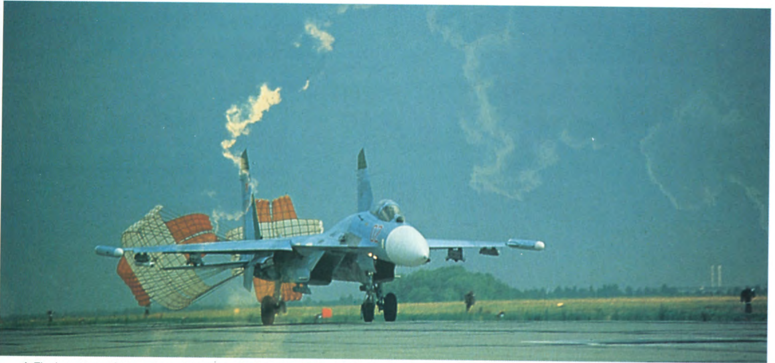
A Flanker returns from a combat training mission. The deployment of its orange-white cruciform chutes reduces landing distance considerably. Note the openness of the Russian landing strip.
