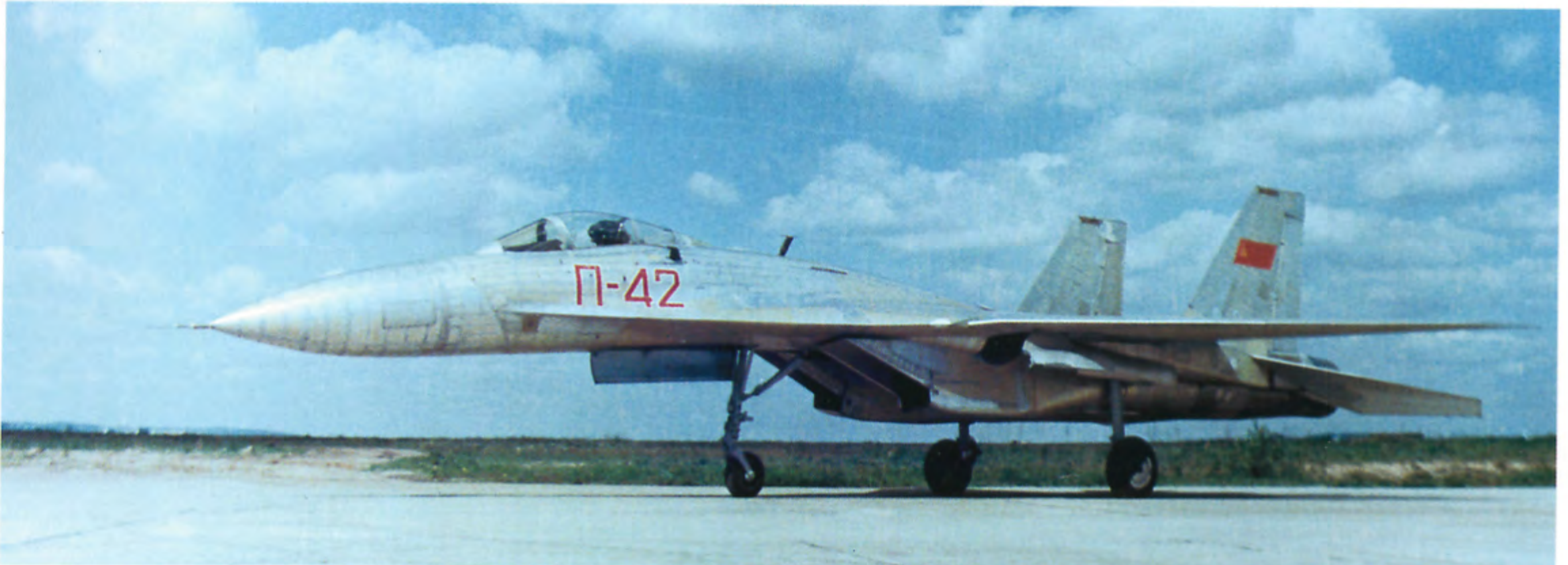
The P-42 record breaker. To reduce the aircraft take off weight, the ventral fins, tail boom, wing and vertical fin tips, weapon hardpoints, and some avionics and equipment were removed. The aircraft was stripped of the paint also. Note the flag of the former Soviet Union painted on the tail fin. (Sukhoi Design Bureau)
