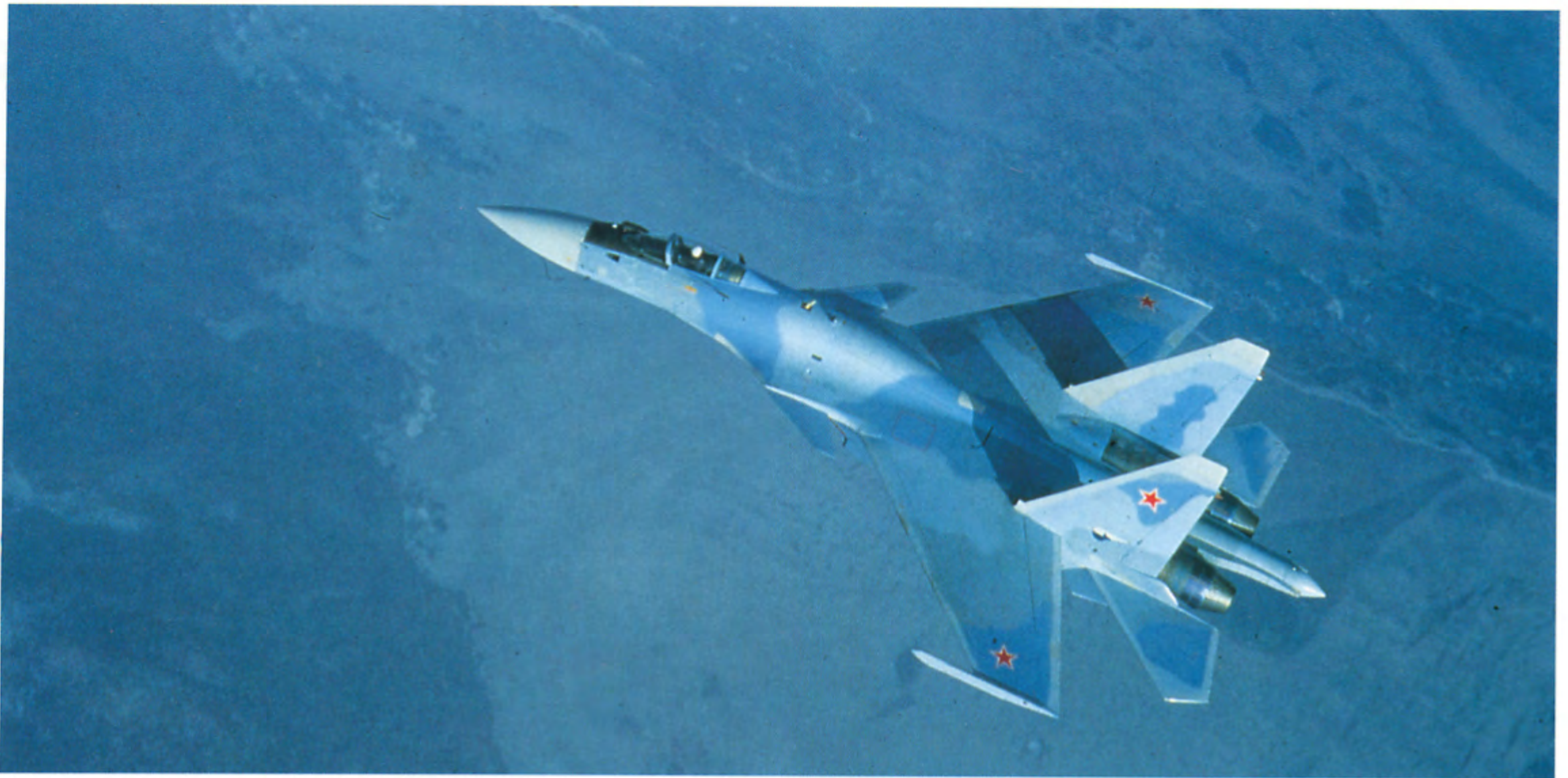
Here a brand new Su-35 overflies the Russian Far East. Its canards are just visible behind the cockpit. These aerodynamic forewings give the aircraft short-field capability and agility.
