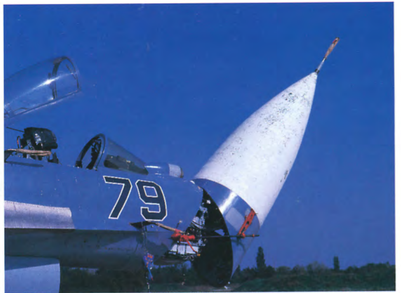
Originally a dazzling white, the radome of Su-27 number "79" is now dirty with use. This workhorse has suffered from the severe, aggressive atmosphere of salt water. The blue paint has held up well in comparison.
