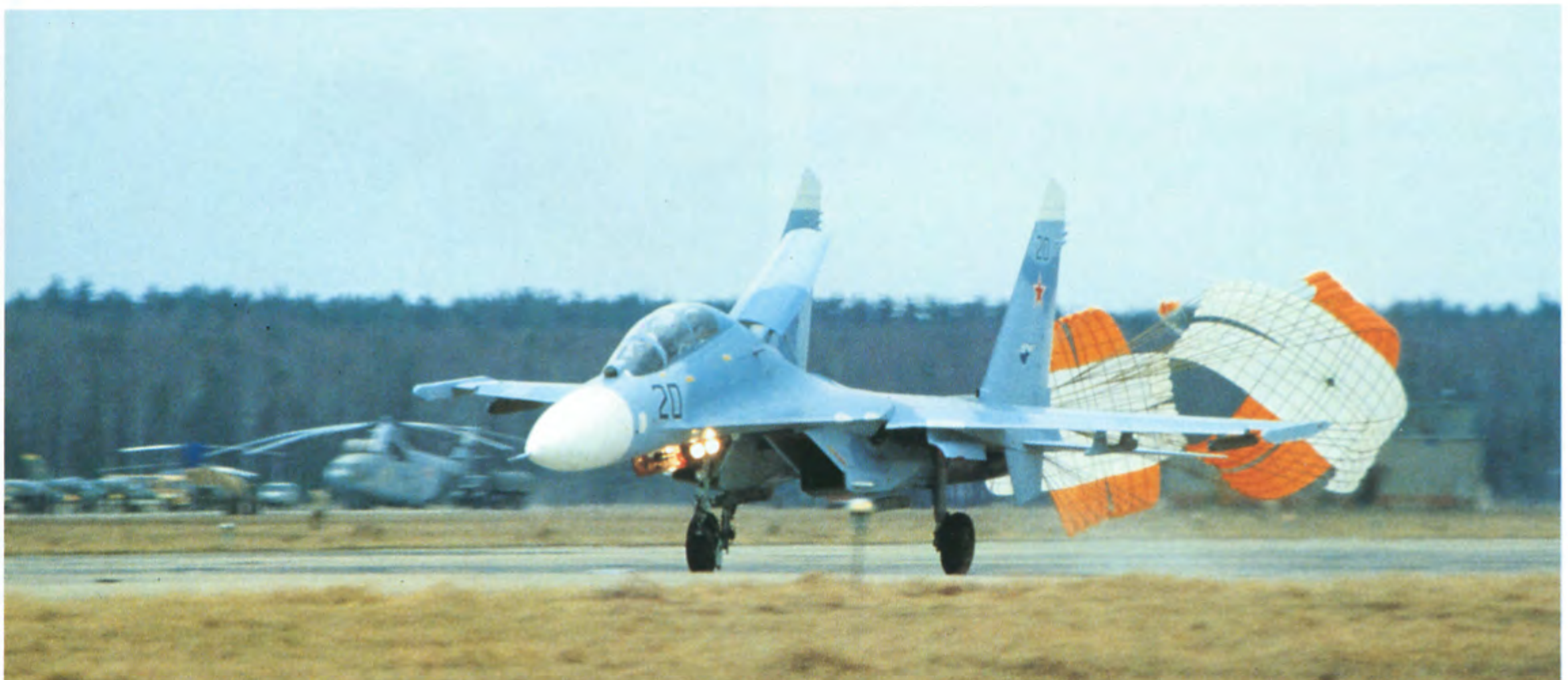
The shape of the Su-27UB dorsal speed brake differs from that of the single seater. Flanker C has also increased area of the empennage. They are basically the same design otherwise.
