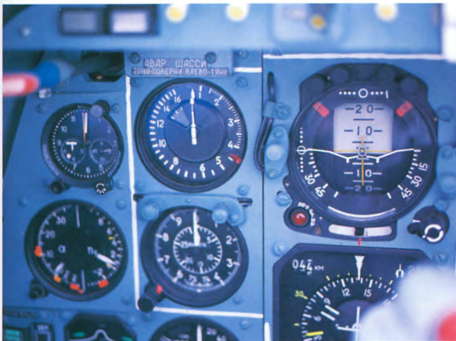
The left side of the main panel contains six instruments: clock, G-load and angle of attacks (AoA) indicator, altimeters, both barometric and radio, attitude directional indicator (ADI) and indicated airspeed indicator.
