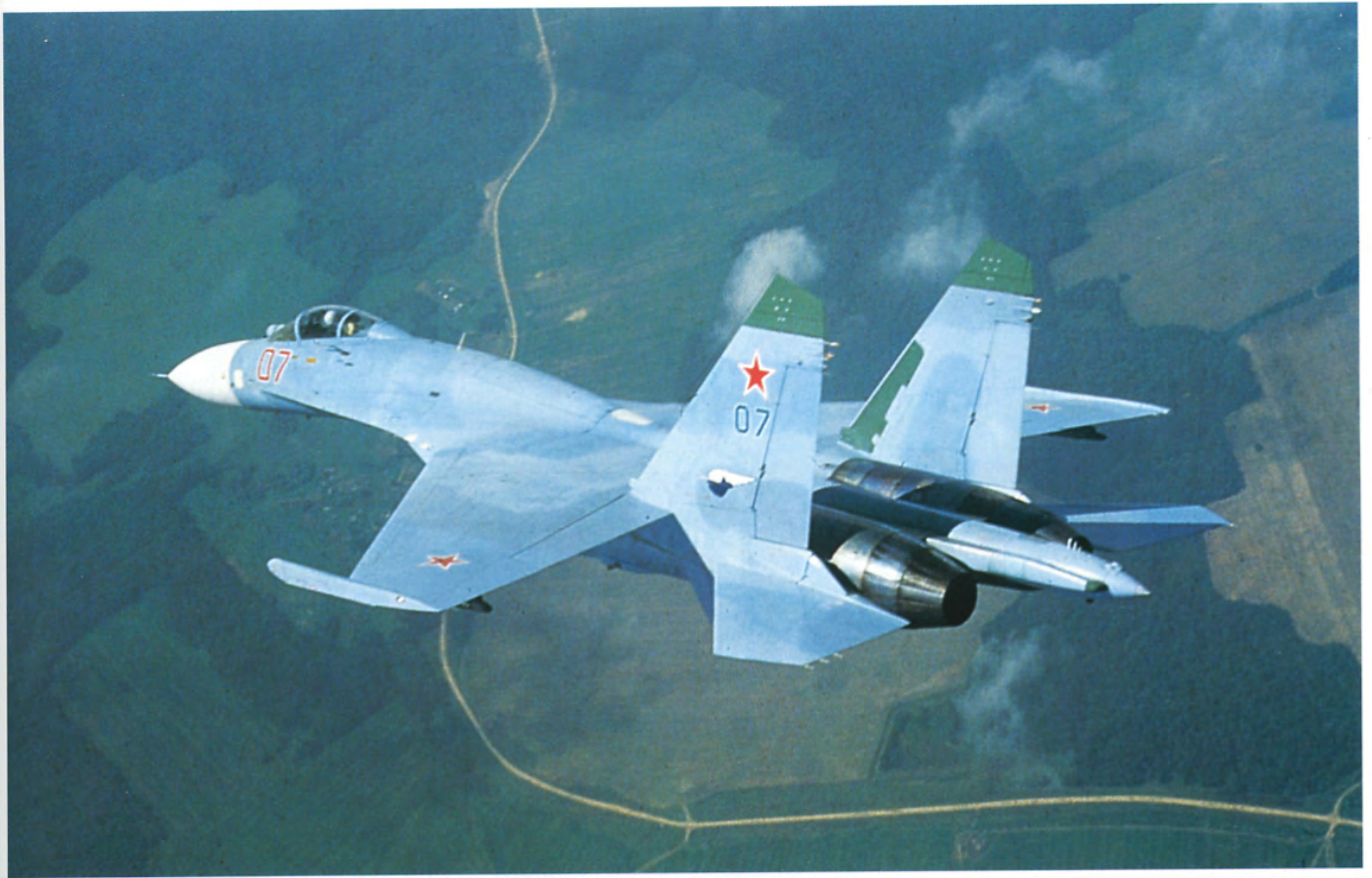
The first prototype of the Su-27 had the wing of Gothic shape. As a result of numerous wind tunnel and flight tests, the Flanker received its tapered swept-back wing with the wing leading edge extension (LEX). This change made a marked improvement in performance.
