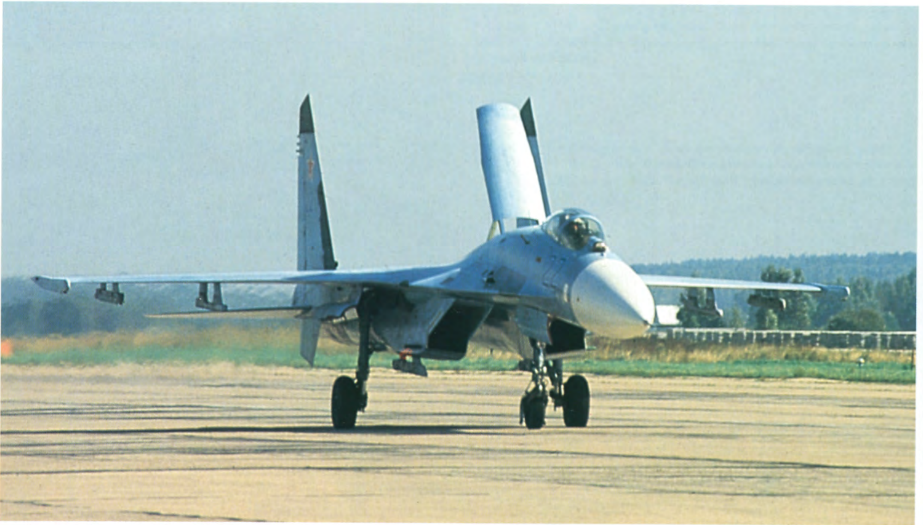
Su-27 landings are frequently made without a drag chute in operational Air Force units. Instead, dorsal airbrakes and wheel brakes are used to moderate extent. Sometimes, the nose is raised to create drag against the underside of the wing.
