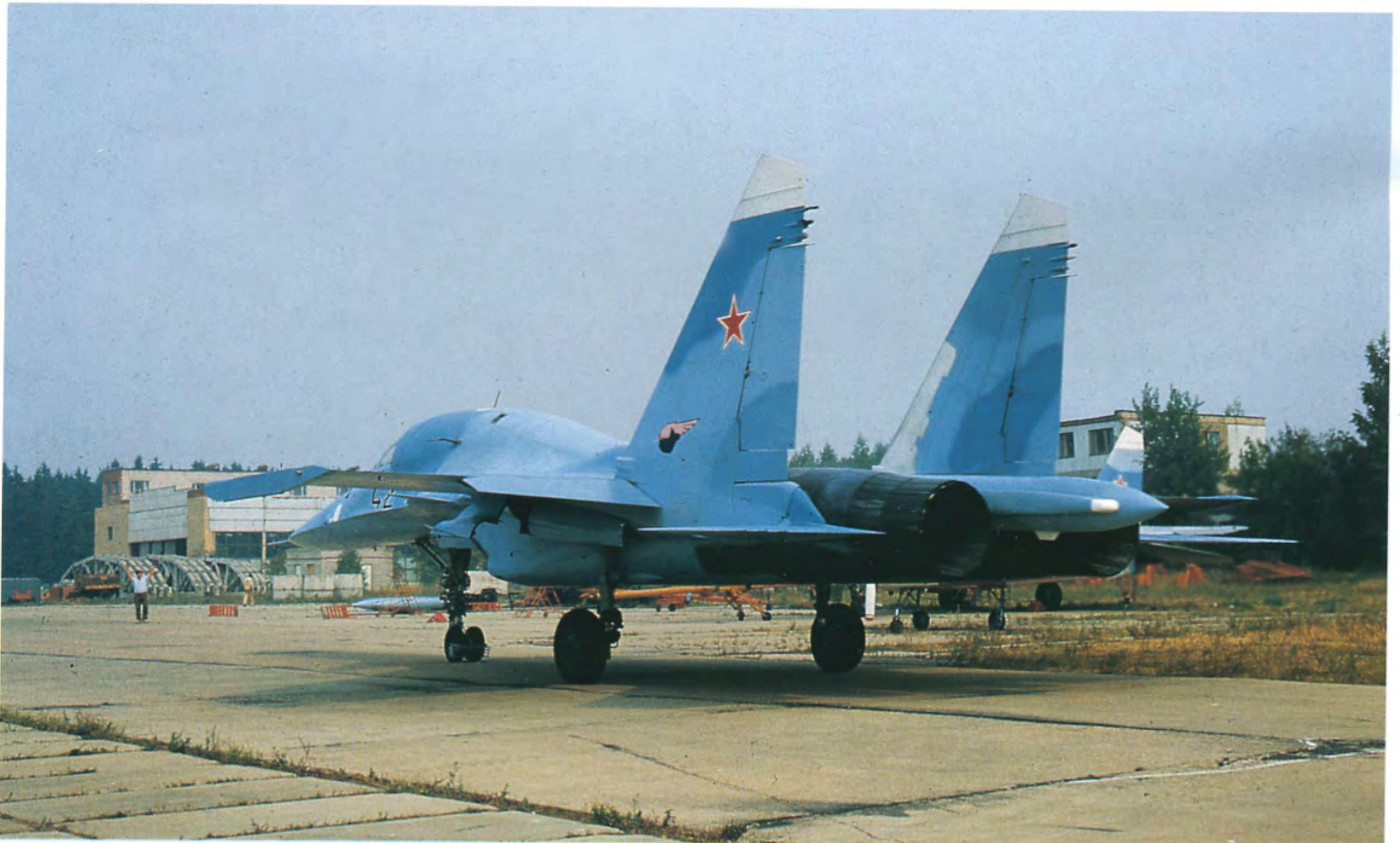
The 35 metric ton Su-27IB has no tailhook. Nevertheless, the claim was made at MosAeroshow that it was capable of being used for training pilots for carrier landing missions. If this is true, it proves an increased versatility for the aircraft.
