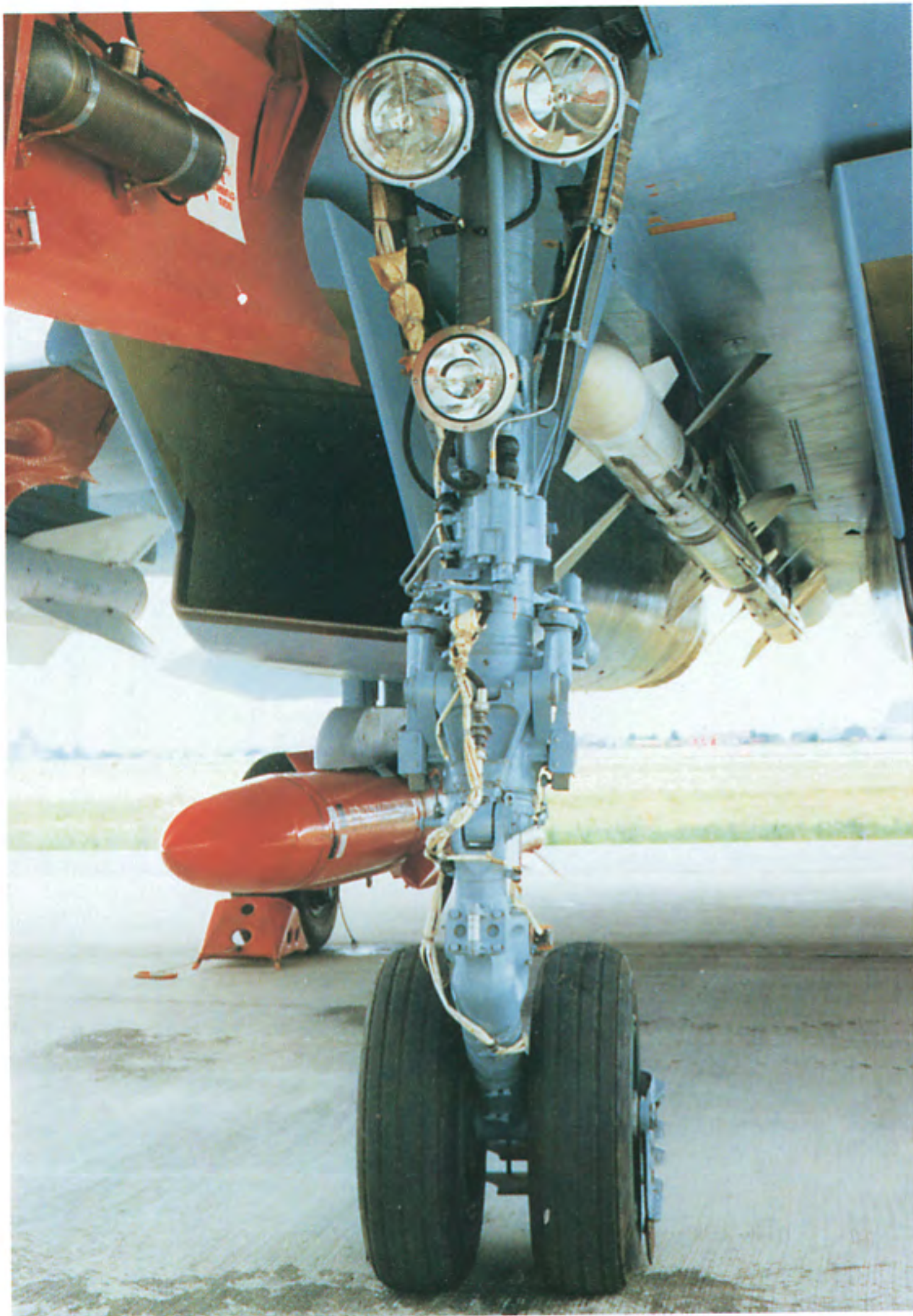
As a departure from the basic design, the Su-35 Super Flanker has a twin-wheel nose gear like the Su-27K. This photo shows the pneumatic reservoir attached to the red-painted panel which powers the nose gear.
