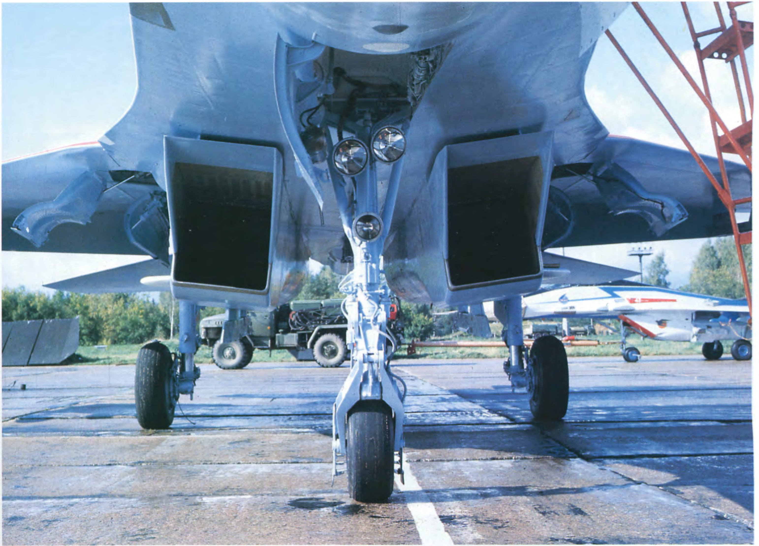
The Su-27 scoop/wing-screened air intakes clearly shown here. Their design provides excellent results throughout a wide angle of attack range. Their squared shape is tapered for improved aerodynamics.
