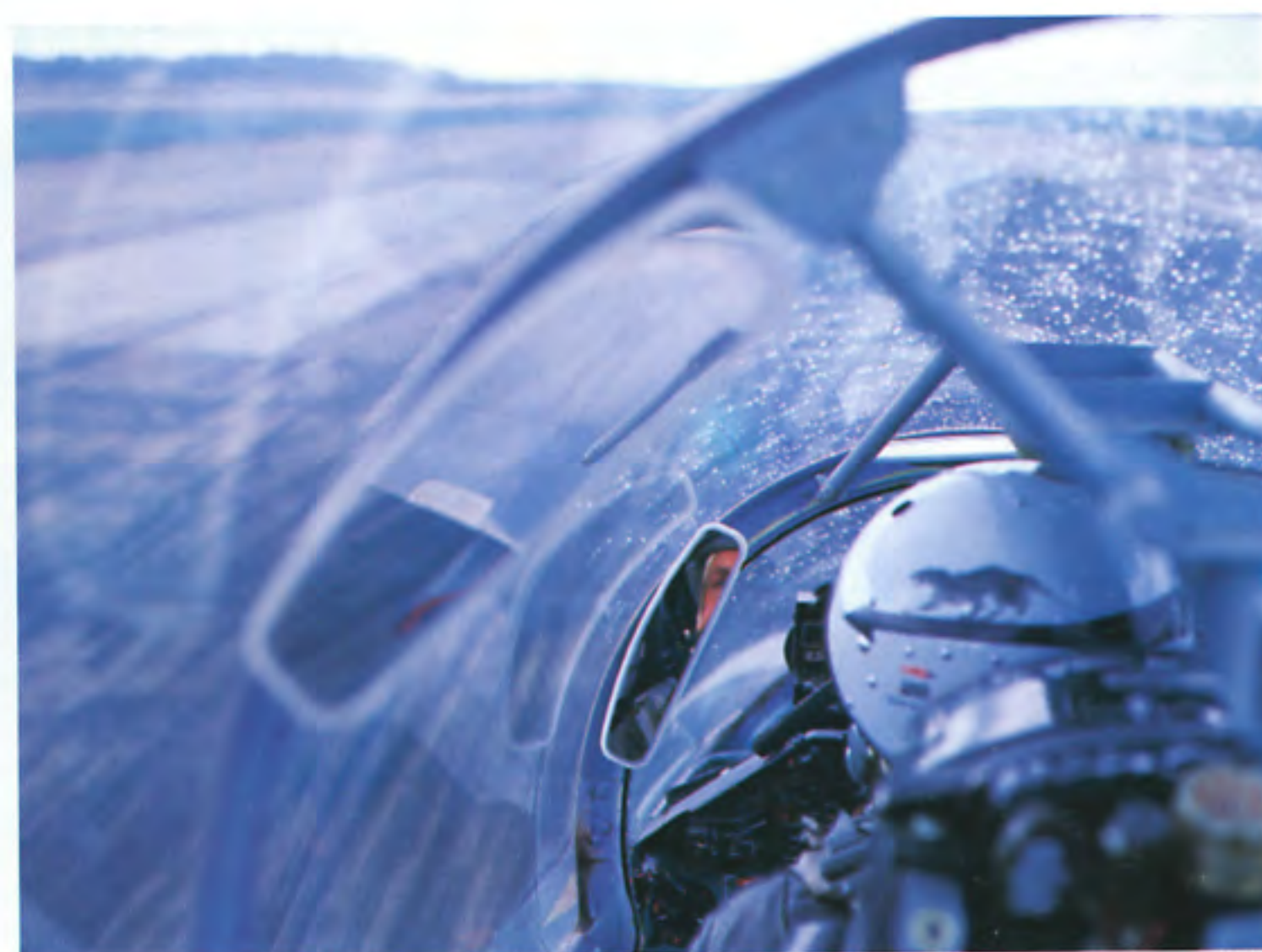
The rear instructor's seat in the Flanker is elevated, unusually for Russian-designed trainers, high above the forward one. The reason for this is made clear by this photo. The forward view from the rear seat is almost flawless.
