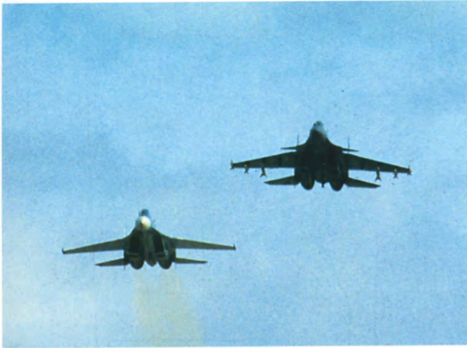
A regular Su-27 and a navalized Su-27 share the sky. The Su-27K distinguishes itself externally from ordinary Flankers mainly by the addition of canards and a tailhook. The canards are barely visible from this distance.
