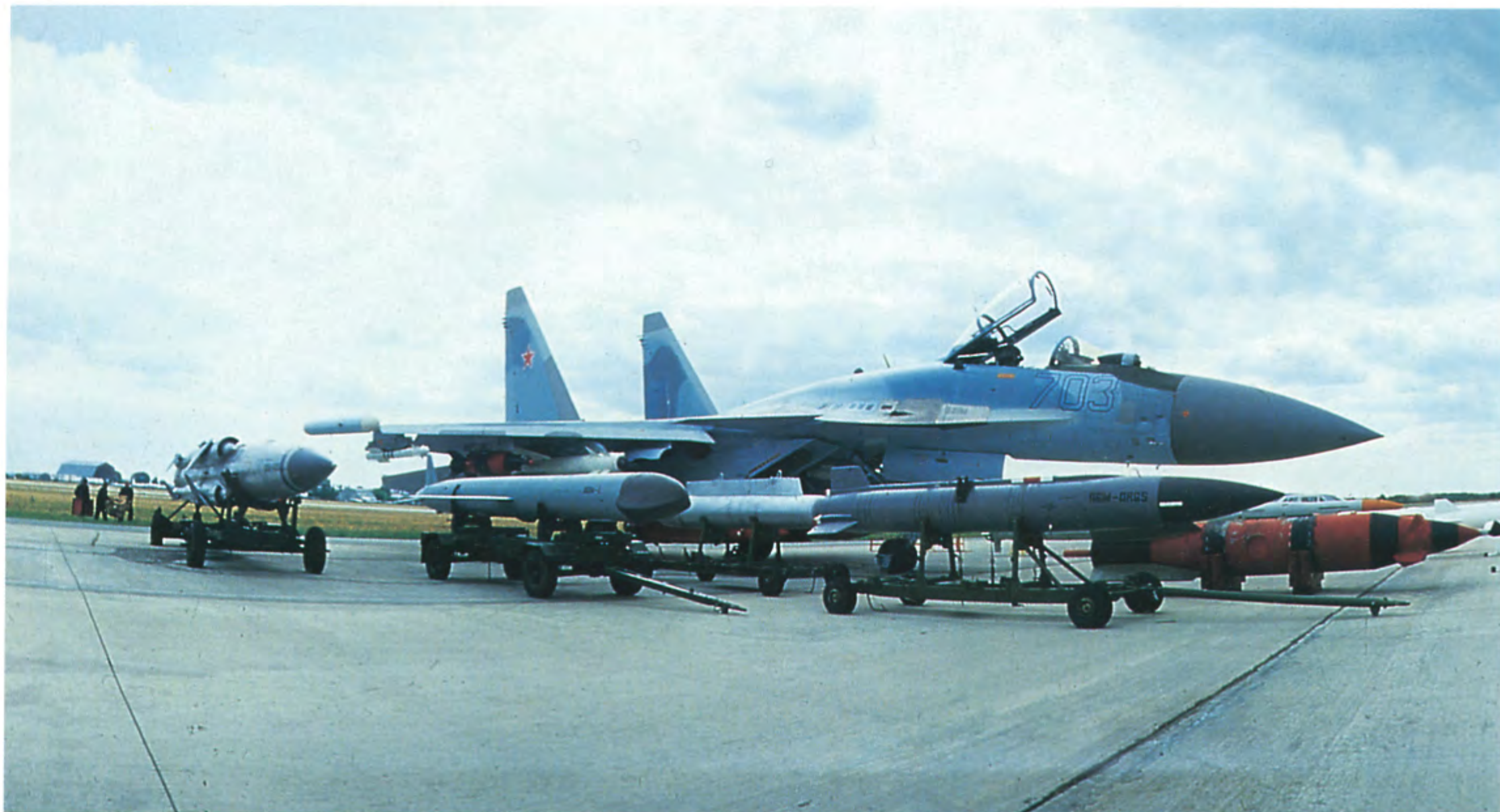
Displayed with its weapons complement is the Su-27M ( modifitsirovanny modified) multi-role fighter. It is designated as the Su-35 by the Sukhoi Design Bureau. The Su-35 reportedly could carry up to 8,000kg payload externally.
