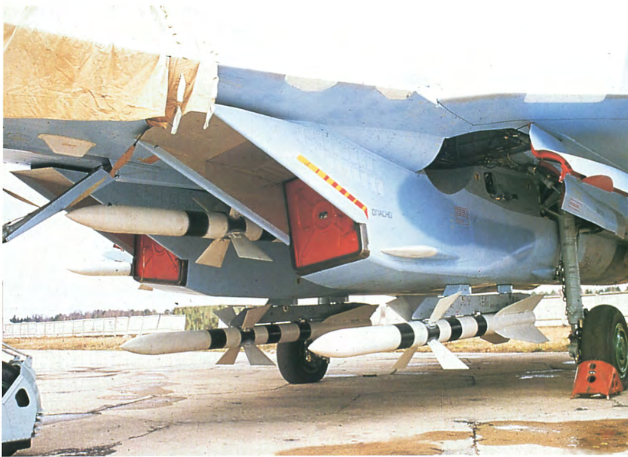
Four radar guided R-27R mid-range AAM in a pair under engine nacelles and another two in tandem between nacelles are capable to engage enemy at medium distance. At the lower left of the picture, the nosewheel mudguard is seen in place. Note also the red engine intake covers. (Yefim Gordon)
