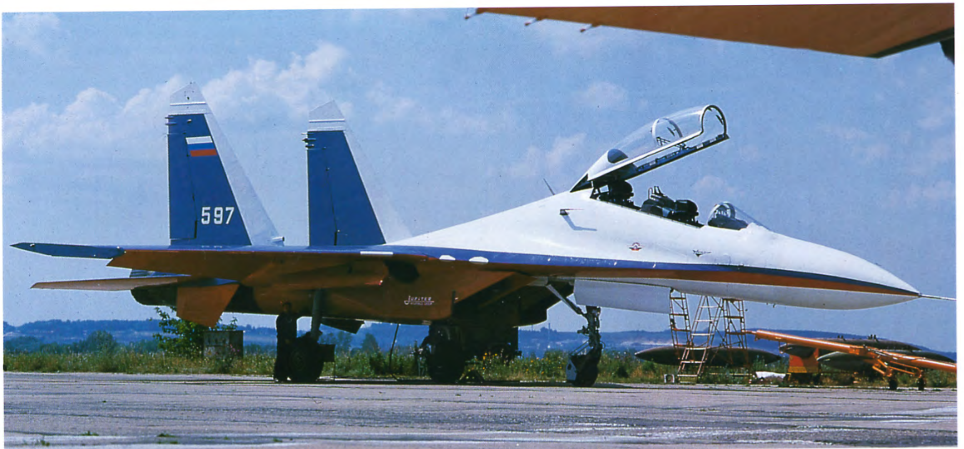
The Su-27PU's cockpit sits high off the ground so access to it is via ladders with attachment hooks above top rung. These ladders are visible on the opposite side of the cockpit. The red undersides of the Flanker is a bright contrast to the traditional camouflage.
