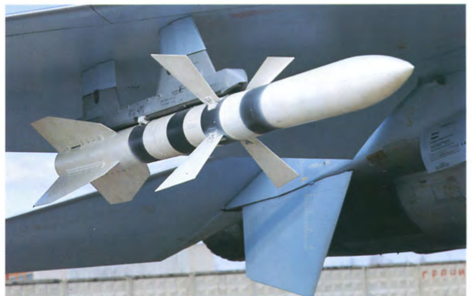
A close-up of an R-27R, NATO codenamed AA-10 Alamo, radar-homing medium range air-to-air practice missile. It is mounted on the APU-470 under-wing launcher of the Flanker. Note its fins.
