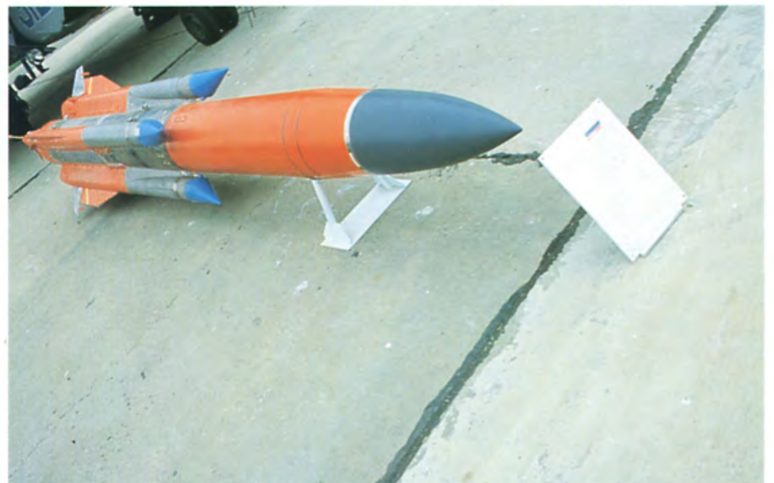
Up to four ramjet powered Kh-31 anti-radiation missiles or Kh-31A antiship missiles can be carried simultaneously by the navalized Su-27K, the new Su-35 and the two-seat Su-27IB fighter-bomber. The missile shown here has an almost toy-like configuration. Those on its receiving end would doubtless disagree with this observation.
