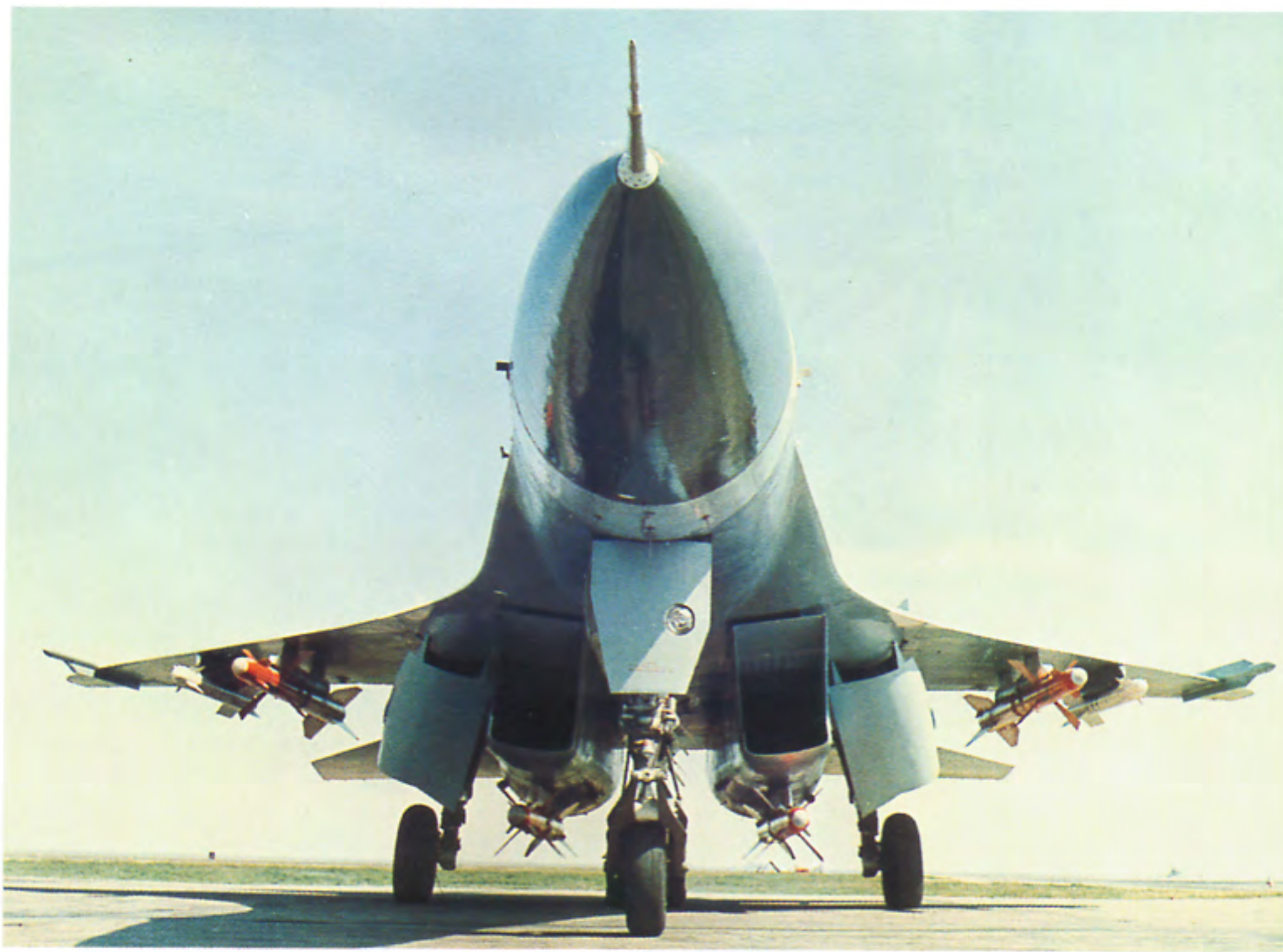
The fifth Su-27 prototype, the T10-5, was used as a testbed for avionics and weapon control system development. The current aircraft still features Gothic wing. Note the placement of missiles under the wings and engine nacelles. Barely visible are the fins of rockets attached between the engines. (Sukhoi Design Bureau)
