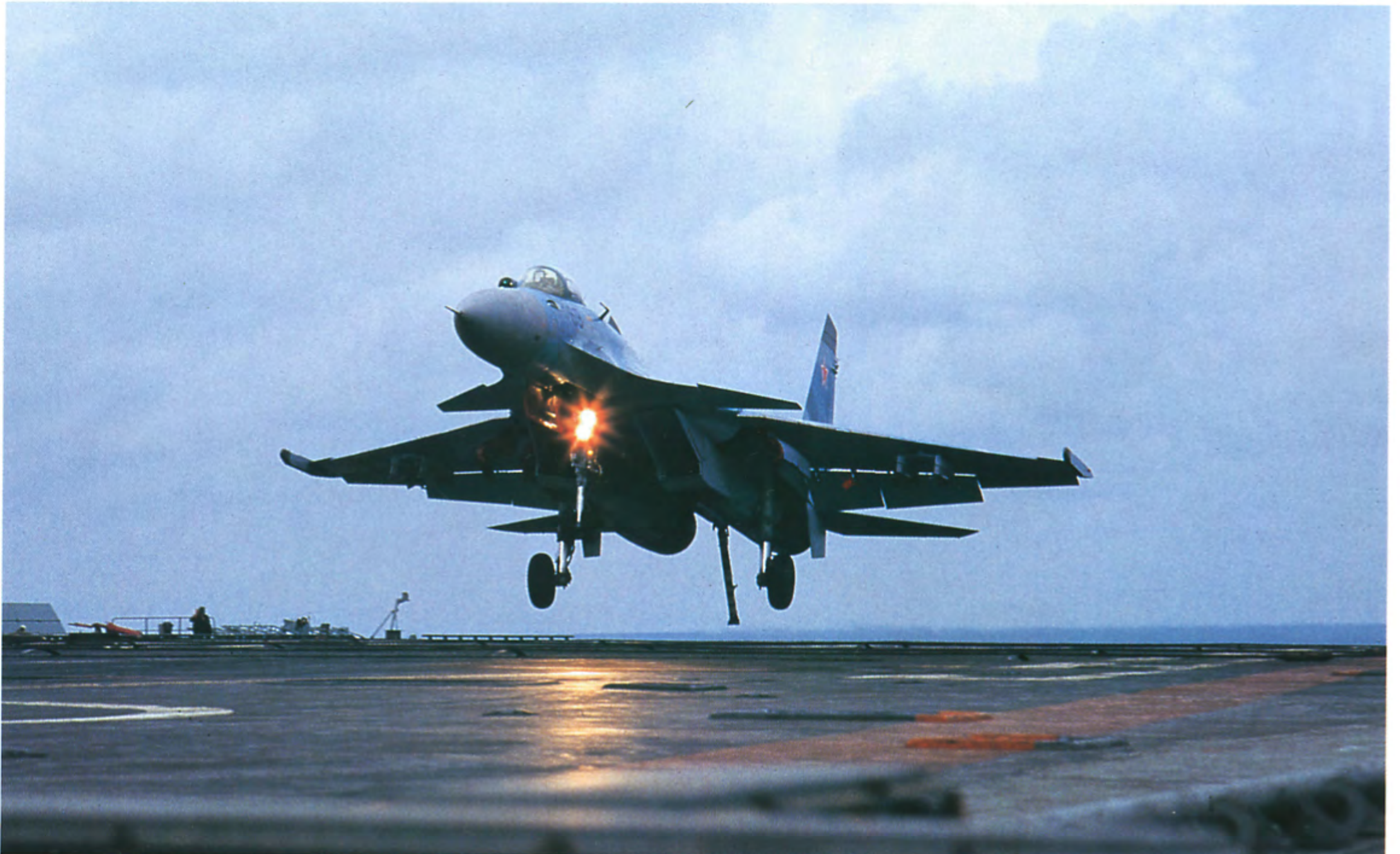
The tailhook of an Su-27K is extended prior to landing aboard the "Kuznetsov" during evening landing practise. As the aircraft lands, the tailhook will catch on the arresting cable. Note the brilliance of the landing lights.
