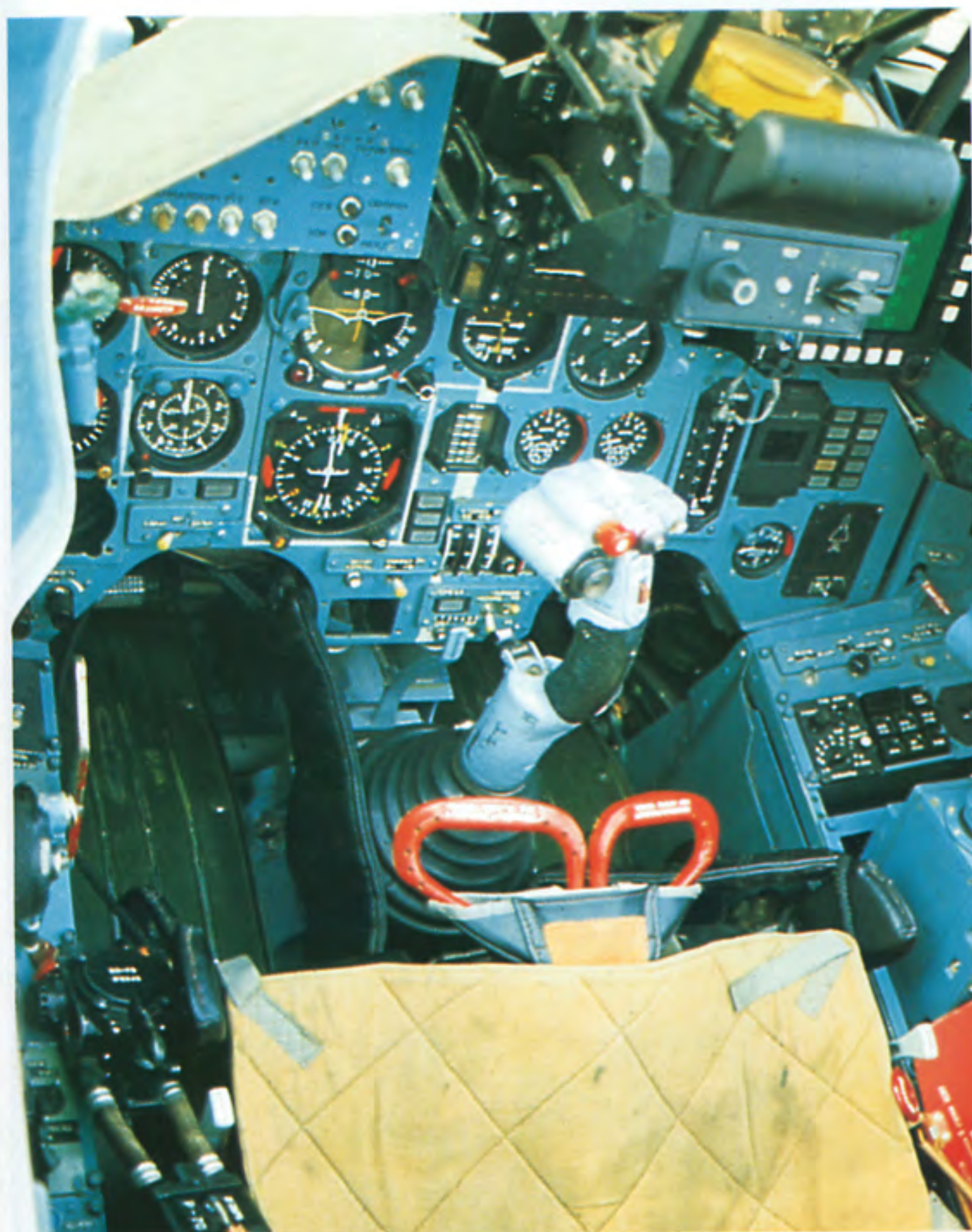
The general layout of the Su-27UB rear cockpit is identical to that of single-seat Flanker. All systems of the two-seater remain the same with the exception of duplicated instrumentation and control. To the novice pilot the array of controls must be mind-boggling. (Yefim Gordon)
