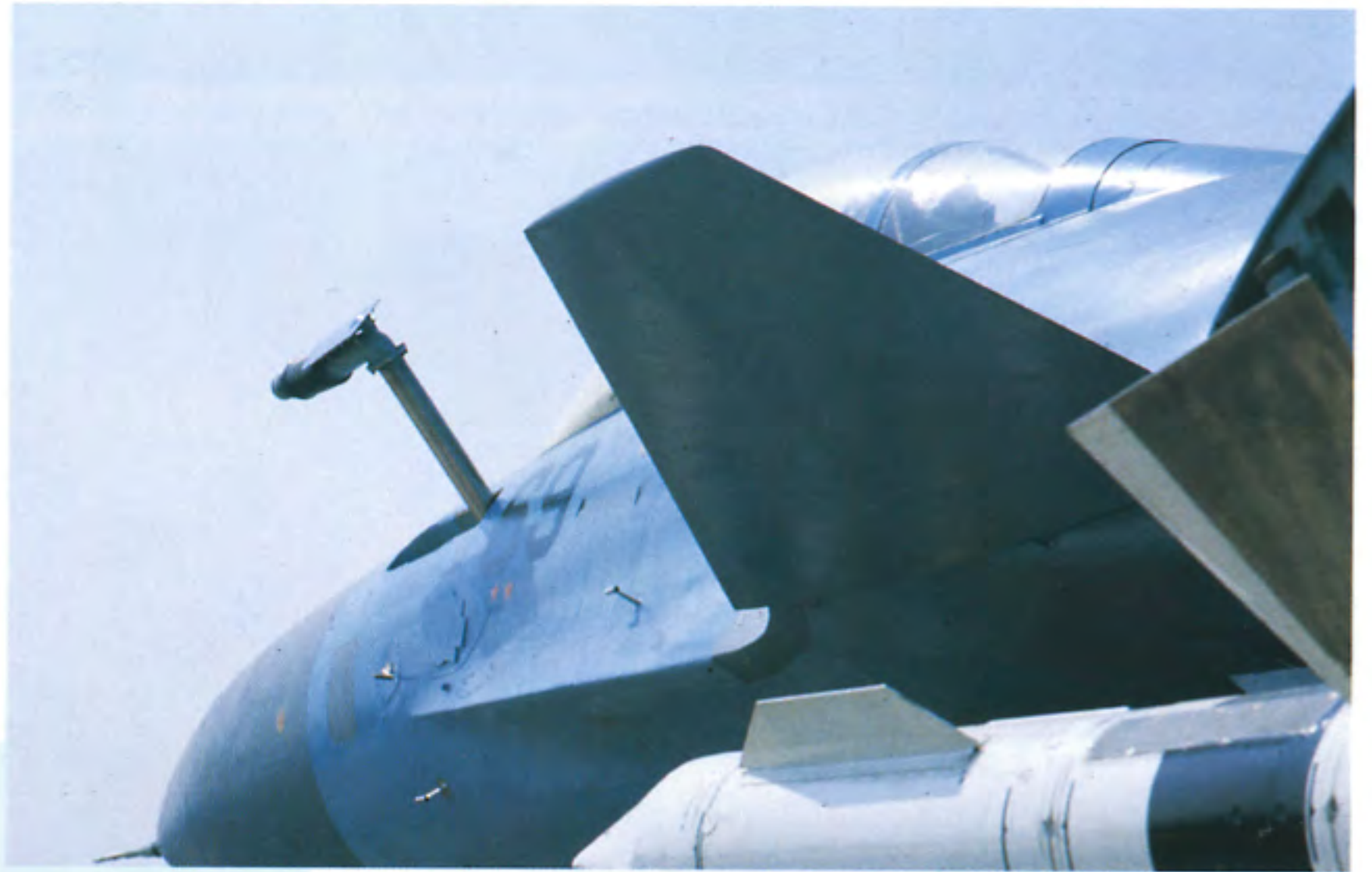
Twelve hard points on the Su-27K allow it to carry a wide range of weaponry from small dogfight AAMs to huge antiradiation and antiship missiles. Notice how the wings of the navalized Flanker are hinged for efficient storage. The in-flight refueling probe protruding from the nose is retractable.
