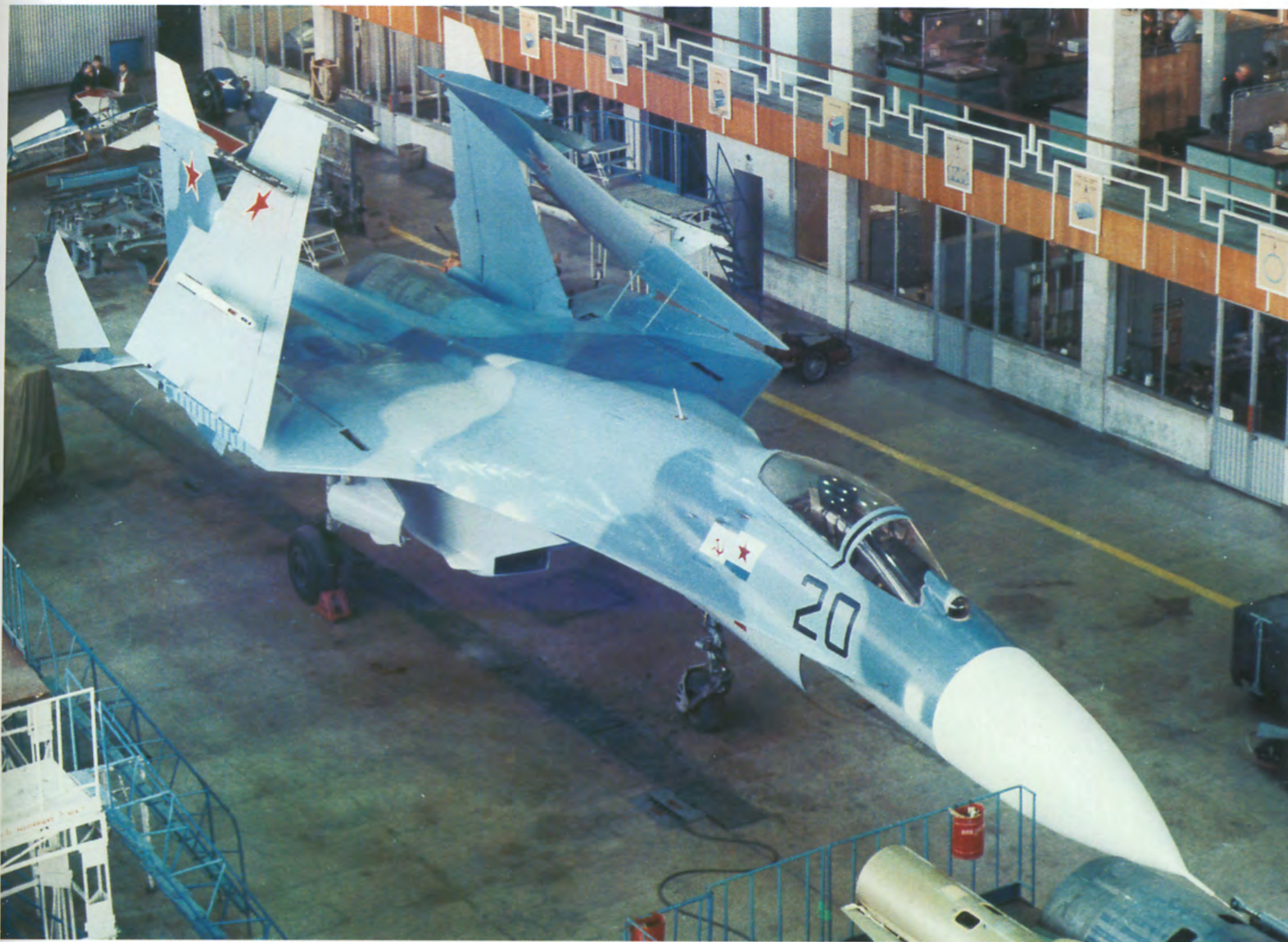
A full-scale mock-up of the navalized Flanker. The lack of the canards, the single wheel nose gear and original position of IRST sensor are noticeable. Note the Soviet Navy Flag beneath the cockpit. (Sukhoi Design Bureau)
