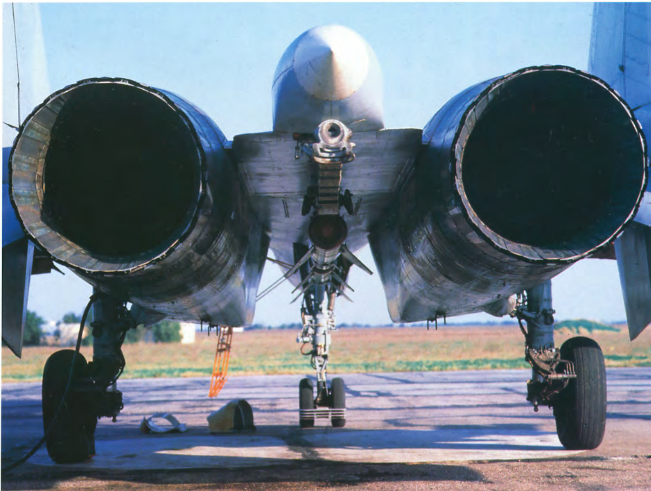
The navalized Su-27 has a strengthened two-wheel nose gear. The three landing/taxiing lights are equipped with LSO (Landing Signal Officer) signal lights. The Su-27K has more pressure in its tires to provide carrier operations with maximum load.
