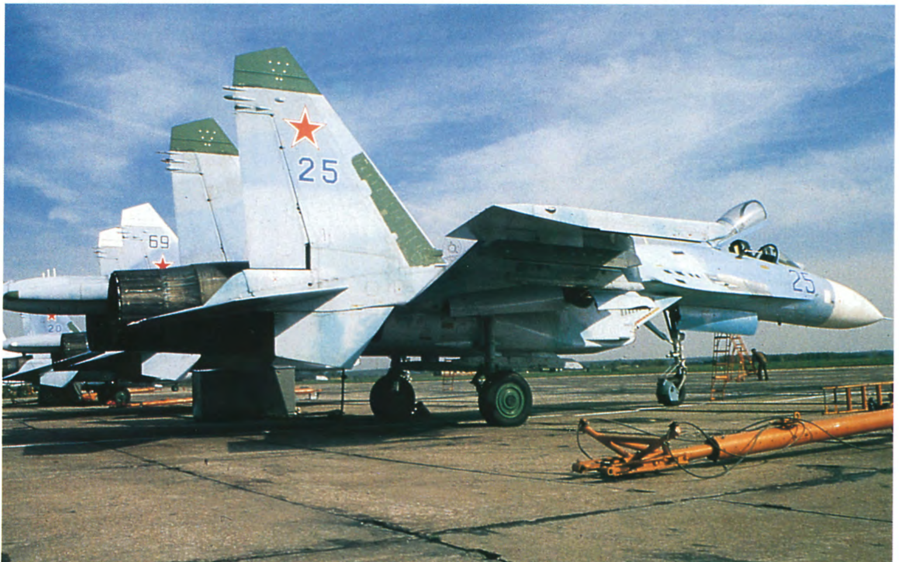
As this photo shows production Su-27 have more spaced fins than the prototypes. Flankers that are in-service are usually painted in the scheme shown here. The dielectric panels and the radomes are either green or white. Both styles appear here. (Yefim Gordon)
