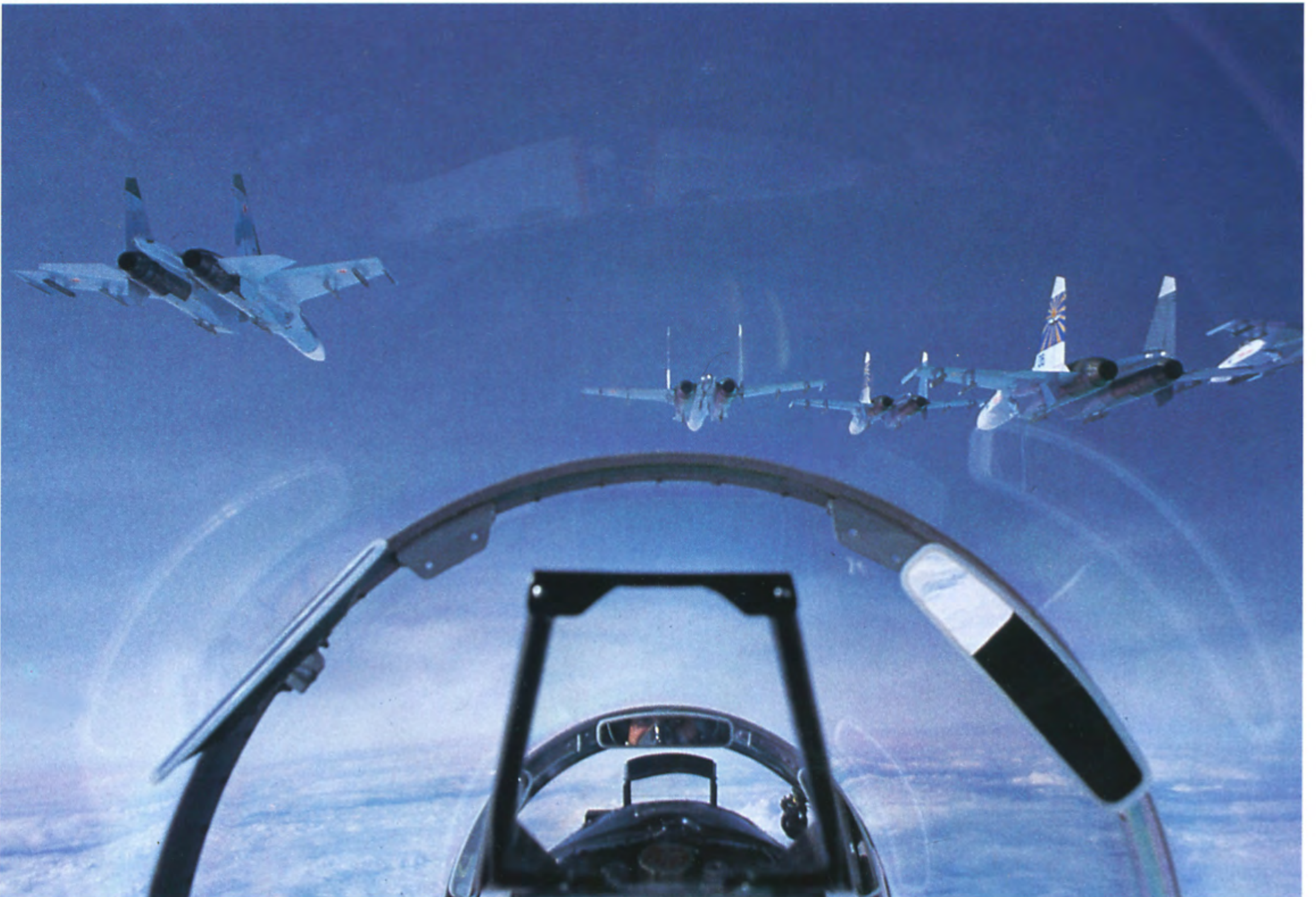
This photograph was taken from the rear cockpit of a Flanker. It gives an idea of the excellent visibility the instructor would have. The lack of obstruction is a tribute to the Sukhoi Design Bureau. (Sergey Pashkovsky)
