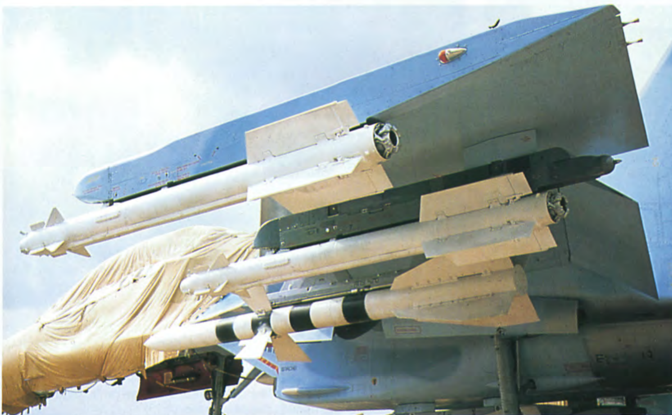
The principal armament of the Flanker comprises medium range radar guided R-27R or IR semi-active R-27T air-to-air missiles. R-73 dogfight missiles (wingtip and outboard mounted) are also employed. This photo shows just how they are mounted to the hard points beneath the aircraft's wing. (Yefim Gordon)
