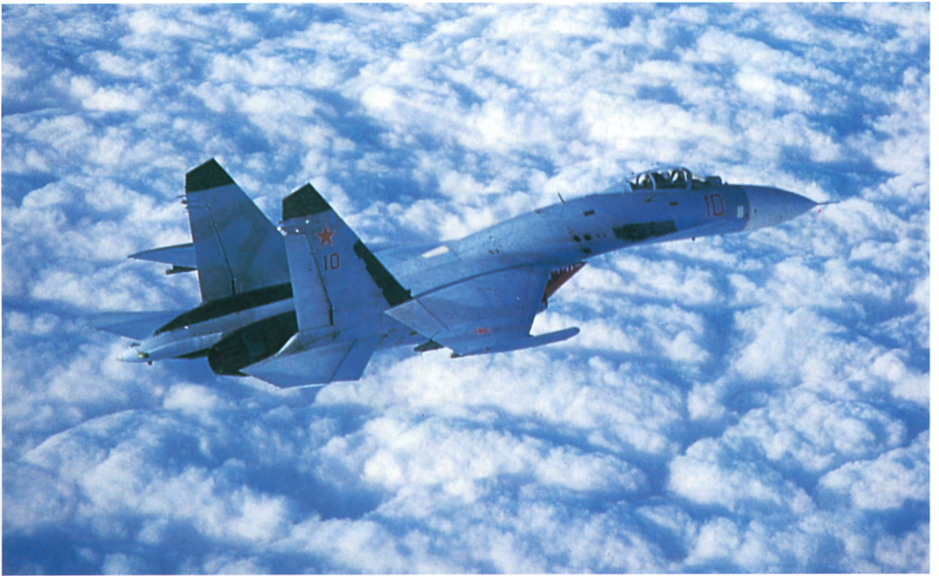
Flanker can intercept targets at heights up to 18,500m. Since the Su-27 was designed to be a long range interceptor, the targets are often beyond visual range. Missiles are provided for elimination of these aircraft.
