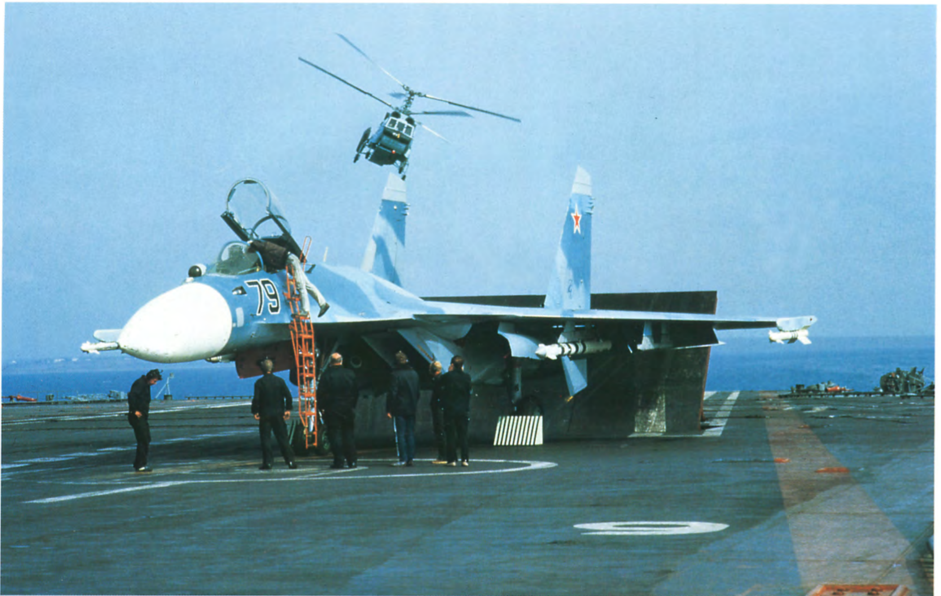
Jet blast deflectors are raised behind Su-27K number "79". They are needed to protect the ground crew and other aircraft from the scorching blast of the engines. Retractable chocks hold the aircraft in place during test runs of the engines.
