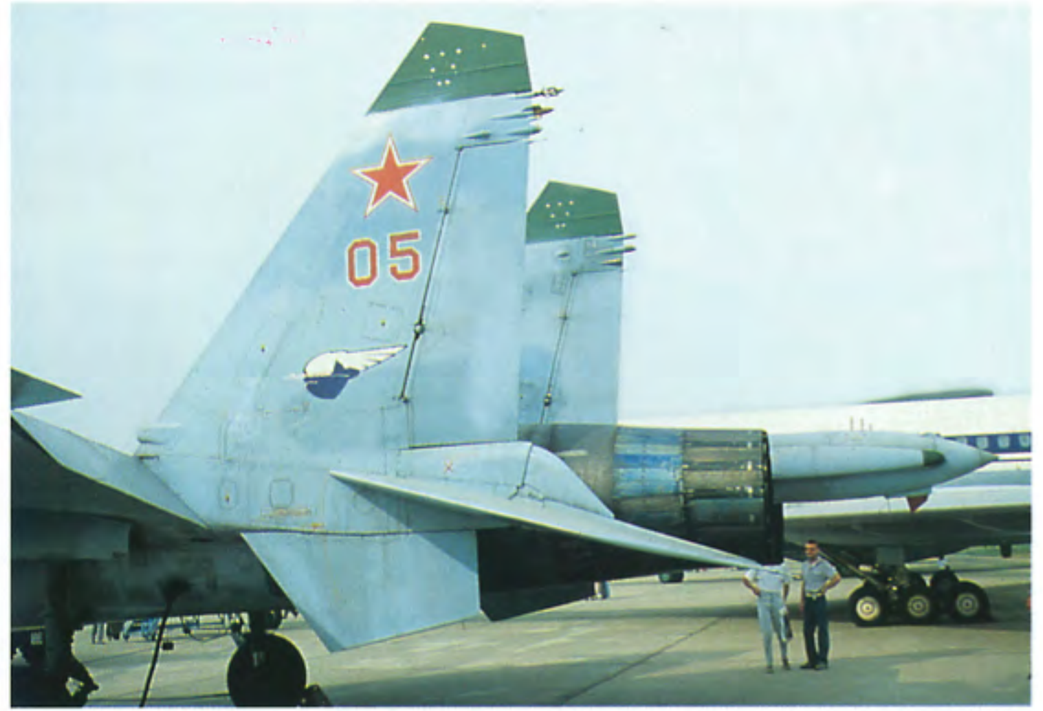
Ventral fins were added to enhance directional stability on high speeds and angles of attack. The long fairing between the engine nozzles is the one that accommodates a drag chute. (Yefim Gordon)
