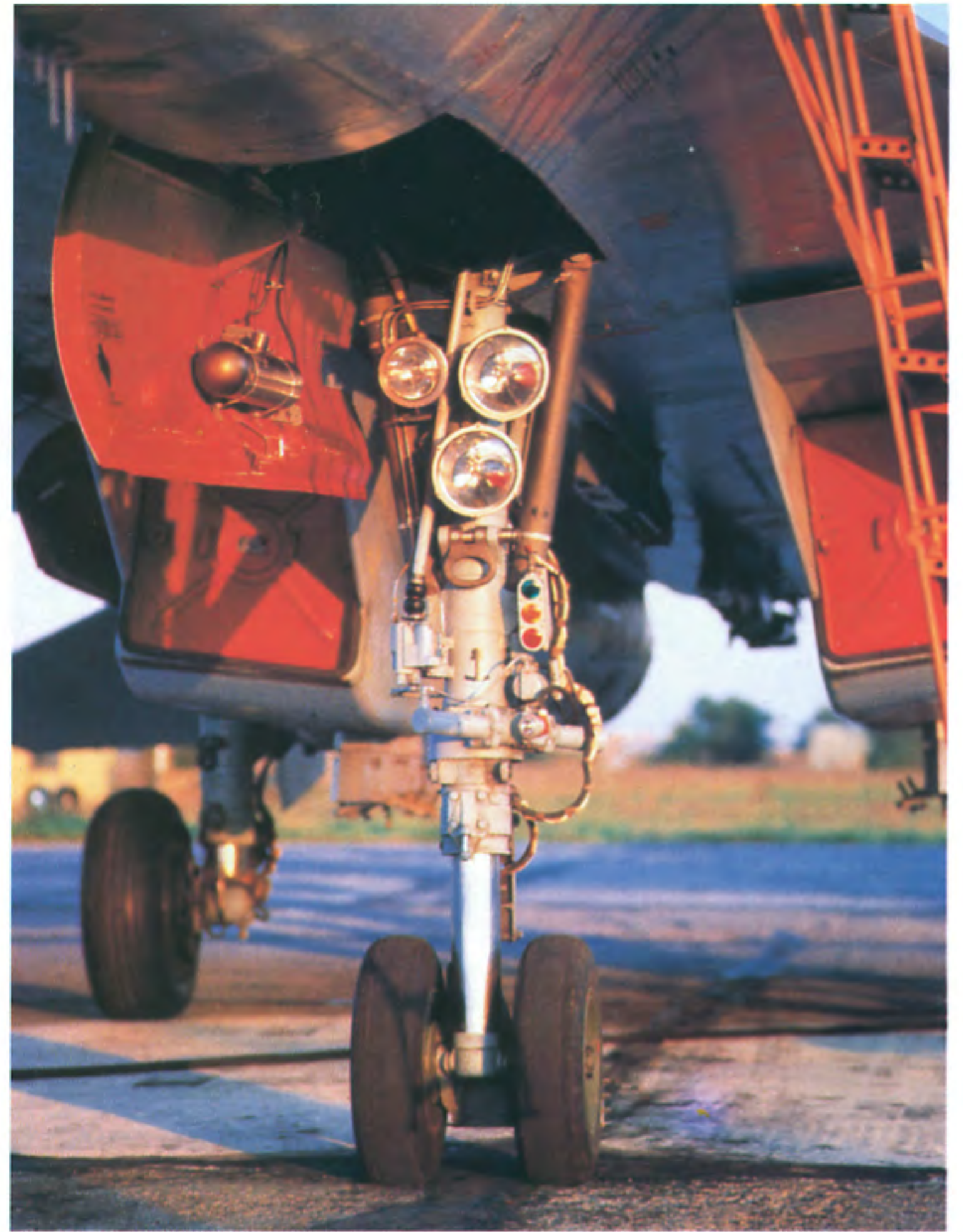
The navalized Su-27 has a strengthened two-wheel nose gear. The three landing/taxiing lights are equipped with LSO (Landing Signal Officer) signal lights. The Su-27K has more pressure in its tires to provide carrier operations with maximum load.
