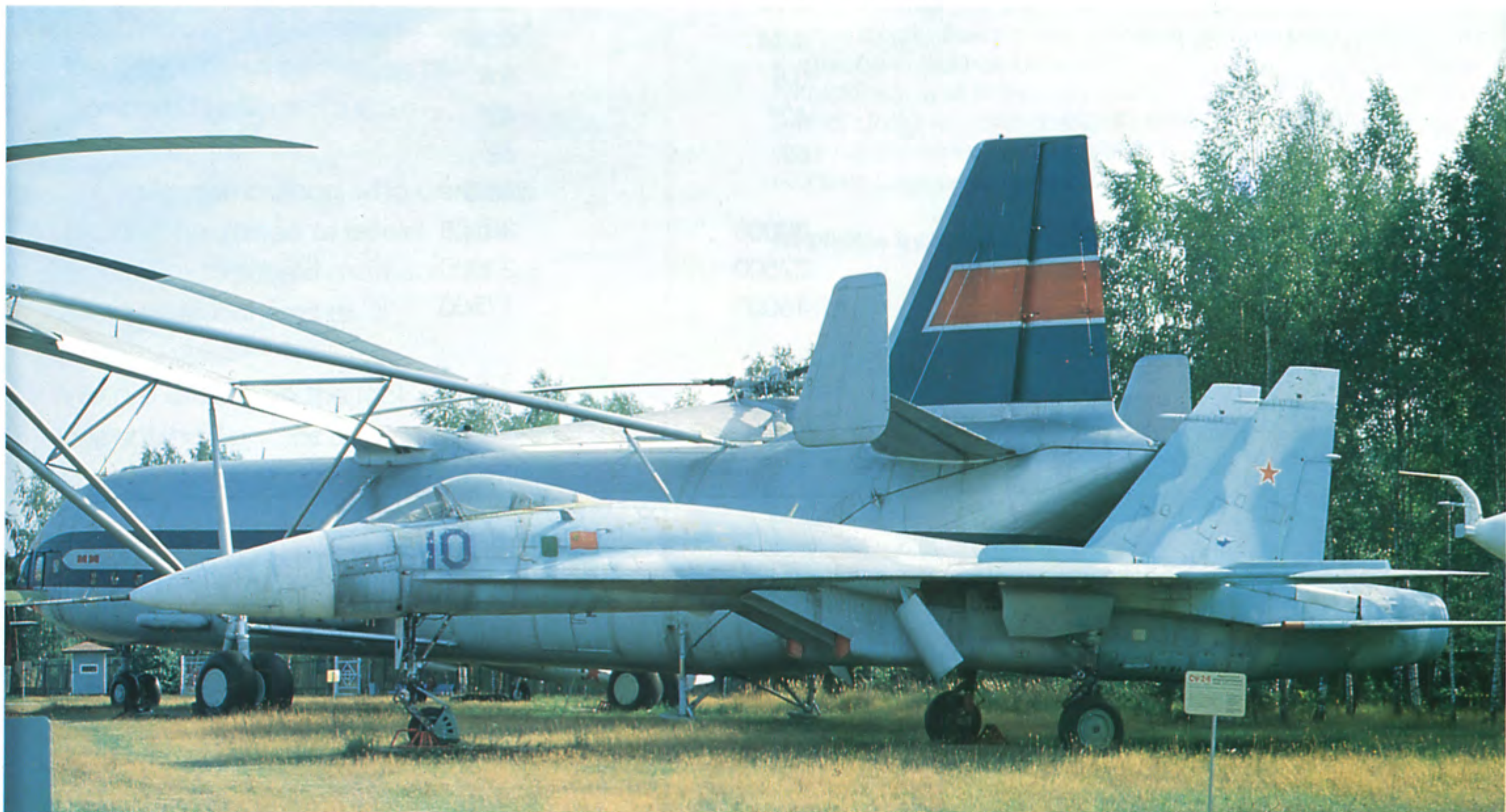
The first Su-27 prototype, designated by Sukhoi Design Bureau as T10-1 (NATO reporting it as codename Flanker A) was used as the aerodynamic testbed for the later production Flanker. Its maiden flight was on May 20, 1977. It is currently displayed at Monino Soviet Air Force Museum. (Yefim Gordon)
