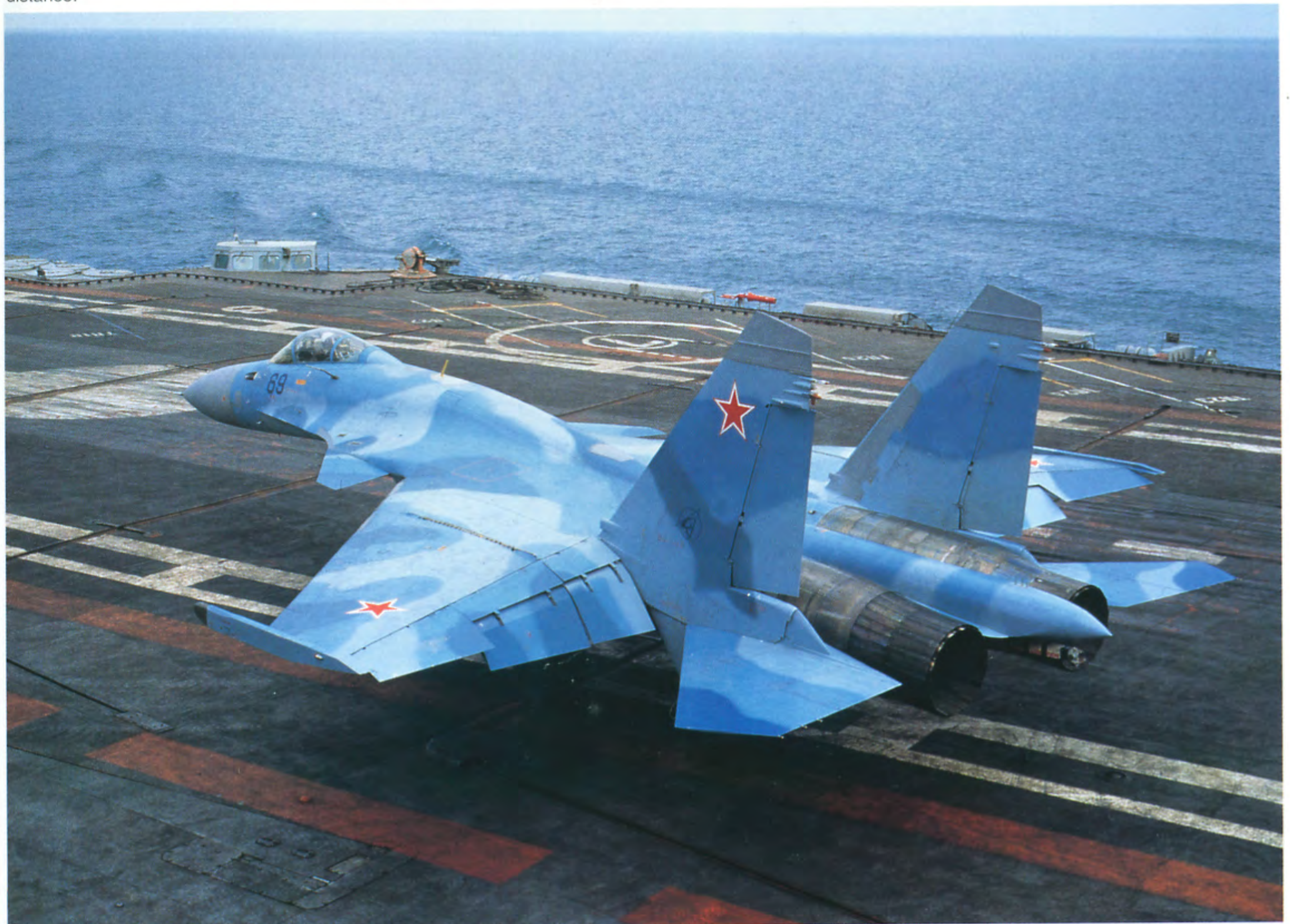
The Su-27K has larger wing platform area. However, the wingspan remains unchanged. Trailing edge control surfaces comprise inboard flaps and outboard ailerons. There is a single flap on the ordinary Su-27.
