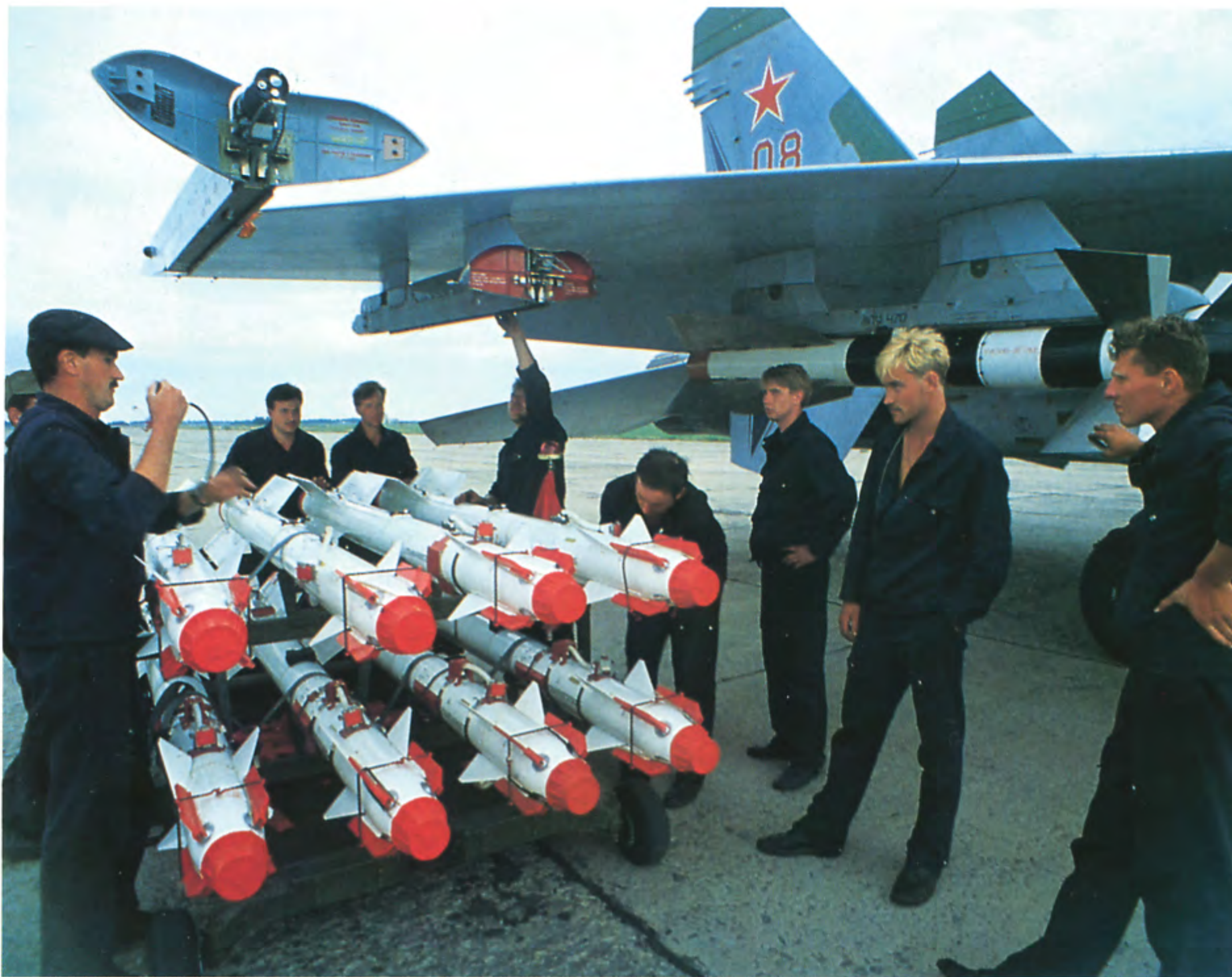
A load of the R-73 missiles sit on the trolley ready for installation on the Su-27 wing stores. Note crocodile-jaw fashion forward parts of missile pylons open. The crowd of young Russian personnel seemed somewhat awed by these explosives.
