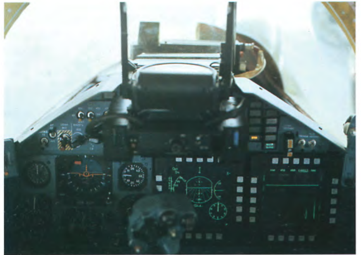
The instrument panel of the Su-35 Super Flanker features two large CRT multi-function displays. It appears to be a more high-tech version of the Su-27's instrument panel. Only a handful of talented pilots ever make use of its dials and switches.
