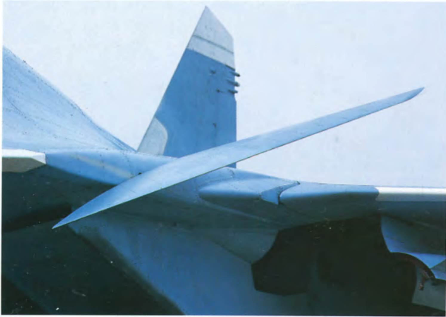
Su-27IB is readily distinguished from other members of the Su-27 family with side-by-side cockpit and the unusual hard-edged front fuselage. The noticeably enlarged dorsal fairing is another new feature. The canards are similar to those used on the navalized Su-27.
