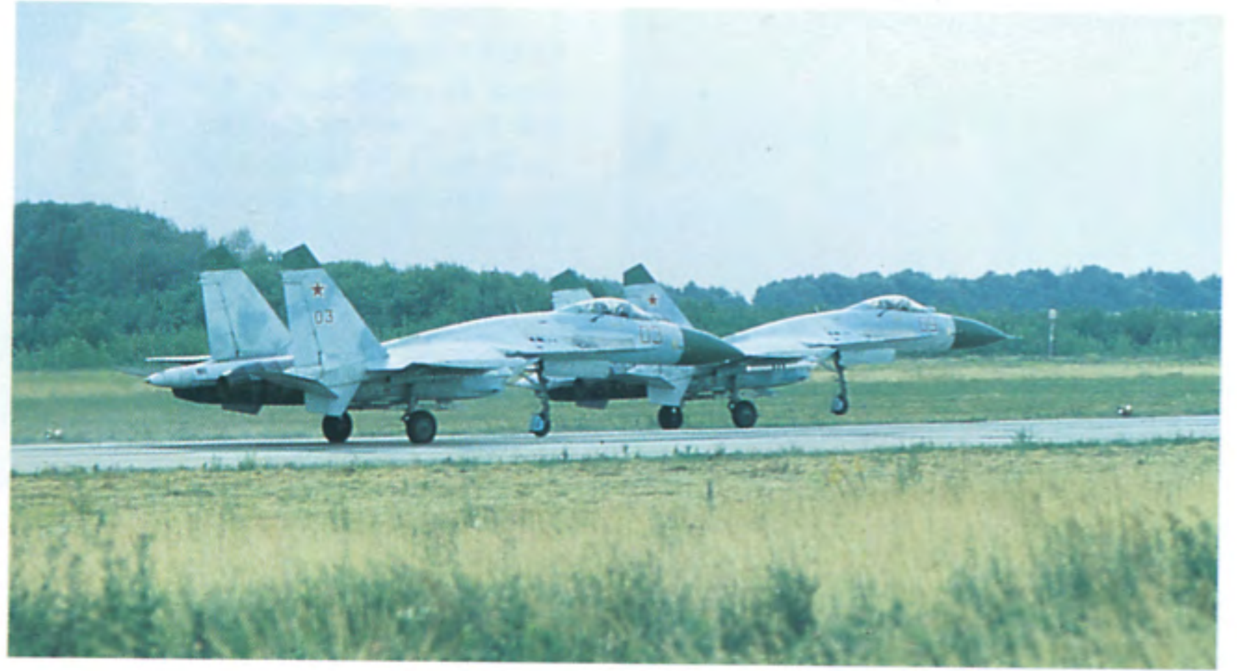
A pair of Sukhoi are ready to get down to business. Note the R-73 (NATO code AA-11 Archer) short range air-to-air missile hinged under wingtip station of leading Flanker. The missiles operate by an infra-red homing system.
