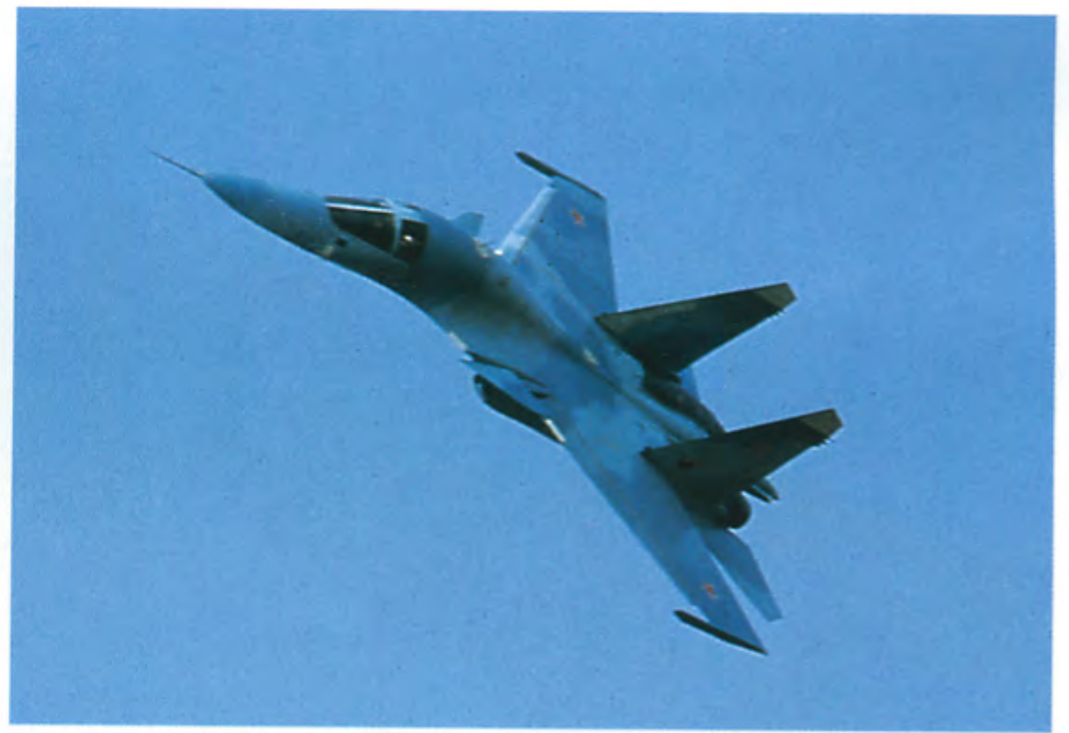
The Su-27IB has excellent performance throughout its flight envelope. This was demonstrated during its display at MosAeroshow in August 1992. Here the canards seem angled somewhat as this maneuver takes place.
