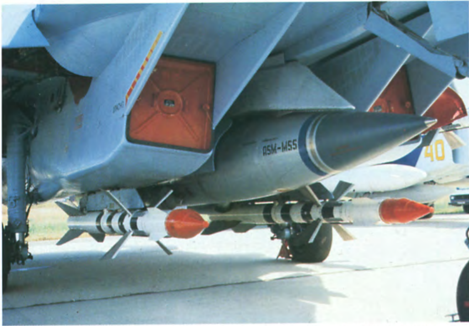
Additional weapon configuration includes AA-10 Alamos under the engine nacelles. An antiship missile designated ASM-MSS is mounted on the belly of the Flanker. It's paint scheme seems elaborate for a missile. (Yefim Gordon)
