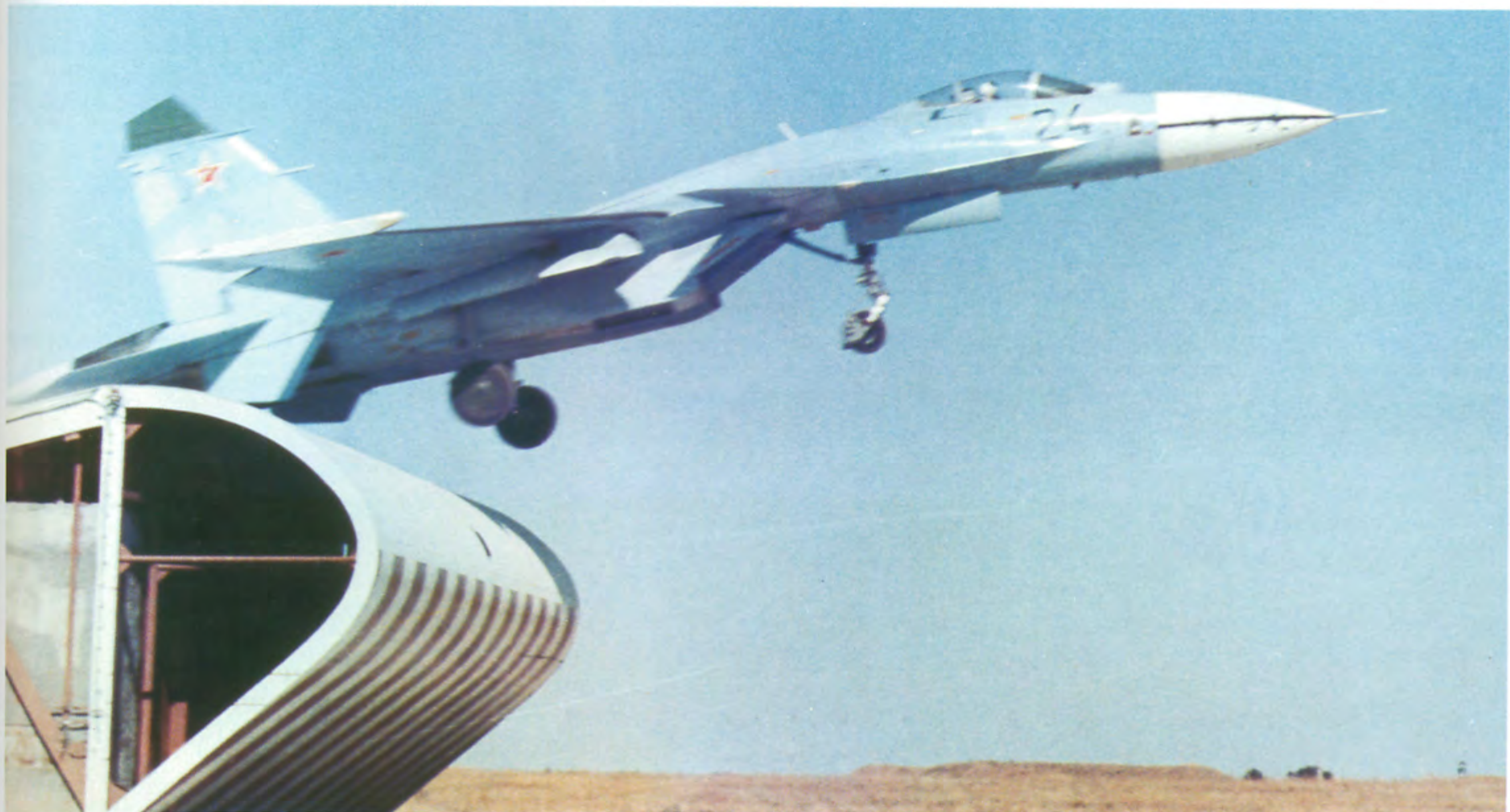
The T10-24 canard-equipped prototype was heavily tested by Design Bureau on ski-jump ramp. To explain the designation number, the "T10" means it is the tenth design with a triangular wing. The number "24" means it was the twenty-fourth one built. (Sukhoi Design Bureau)
