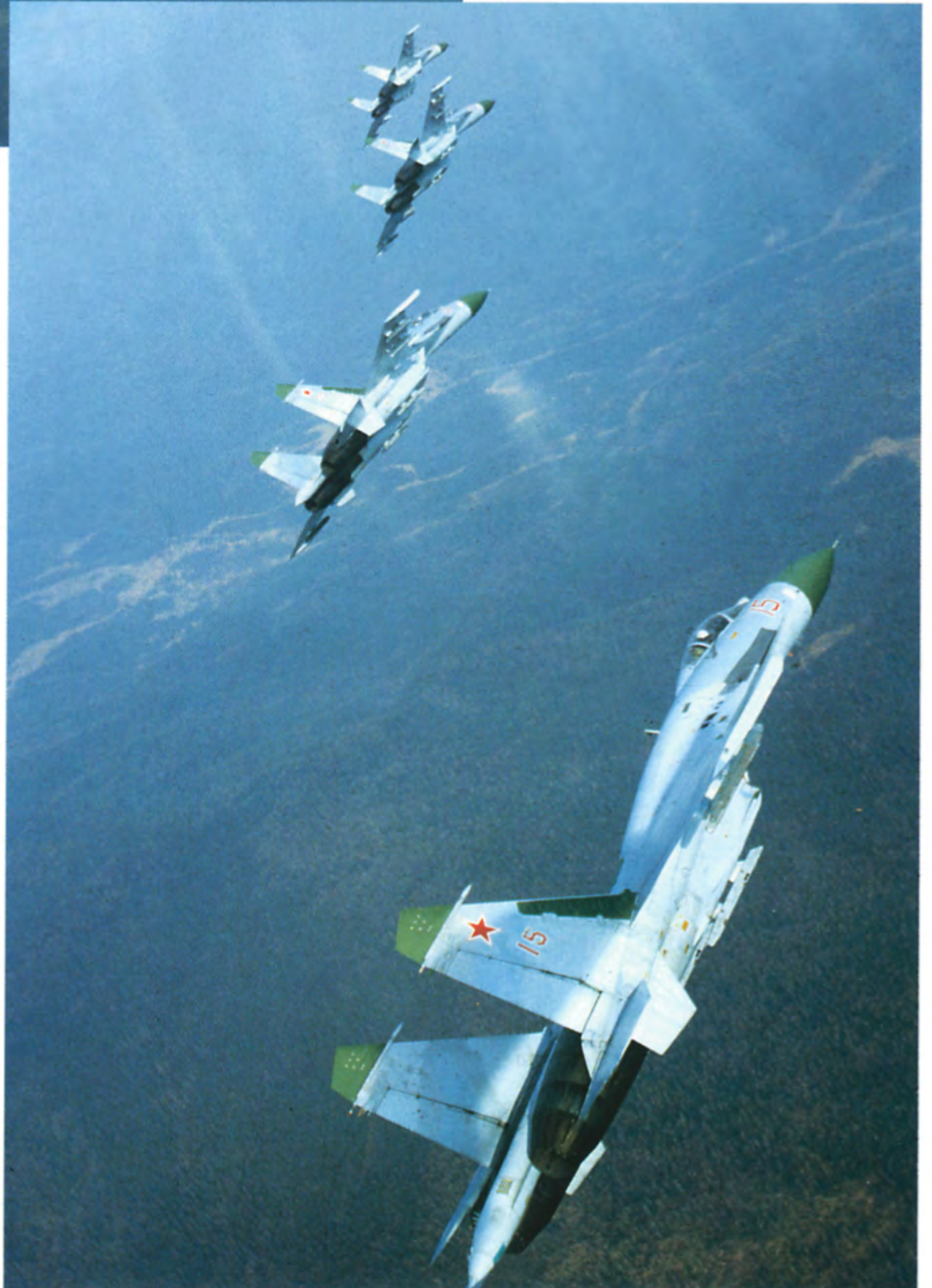
A group of Su-27s painted in standard VVS ( Voennovozdysnyye Sily - Air Force) markings. They are equipped with the dark green radome and dielectric fairings. The precision of their formation flight is noteworthy.
