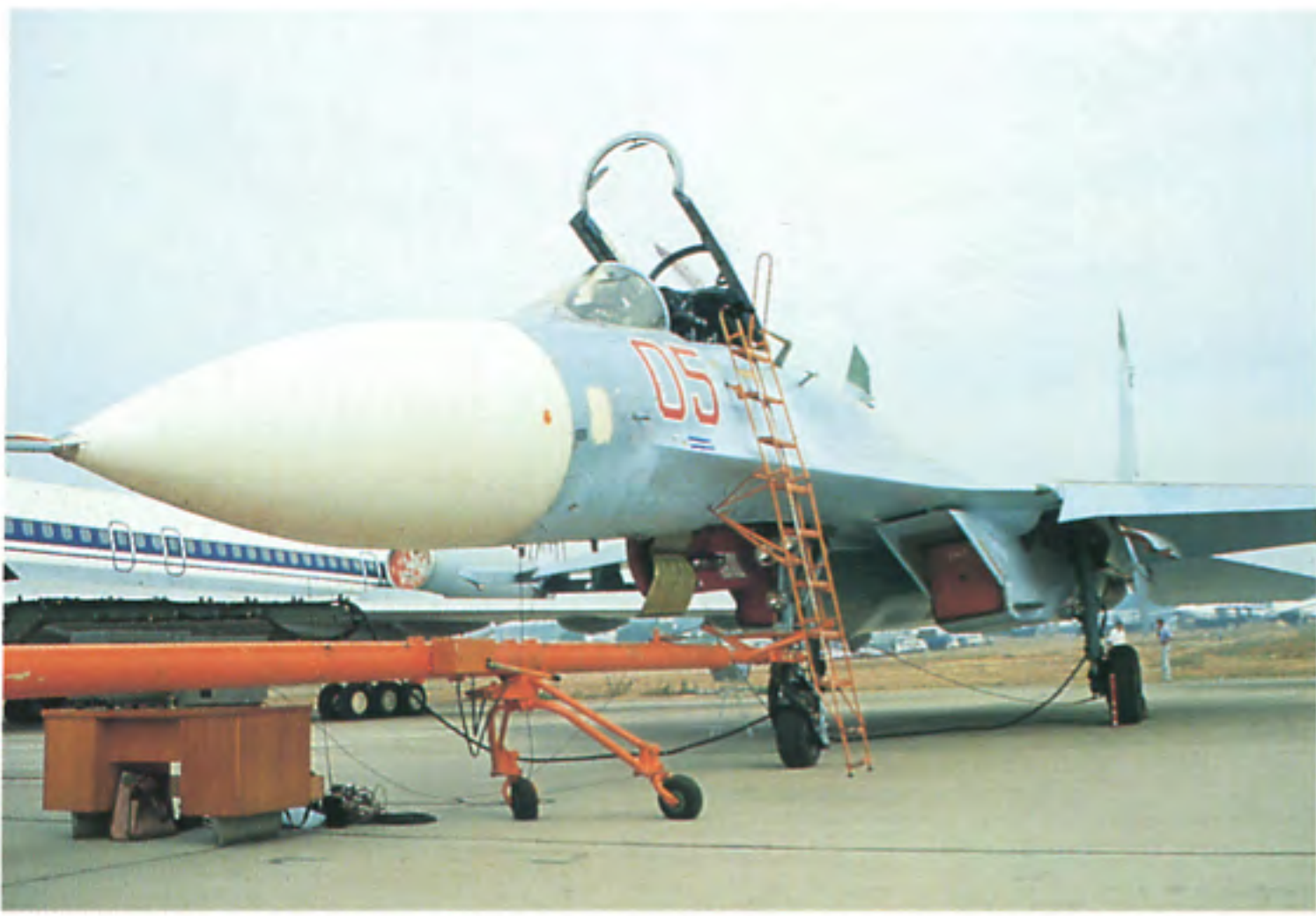
"Red 05" is the Su-27 test aircraft of Zhukovsky LII Flight Research Institute. The aircraft lacks the IRST (Infra Red Search and Track) device. Note the protective air intake covers installed to prevent fatal injury to pilot and ground crew. (Yefim Gordon)
