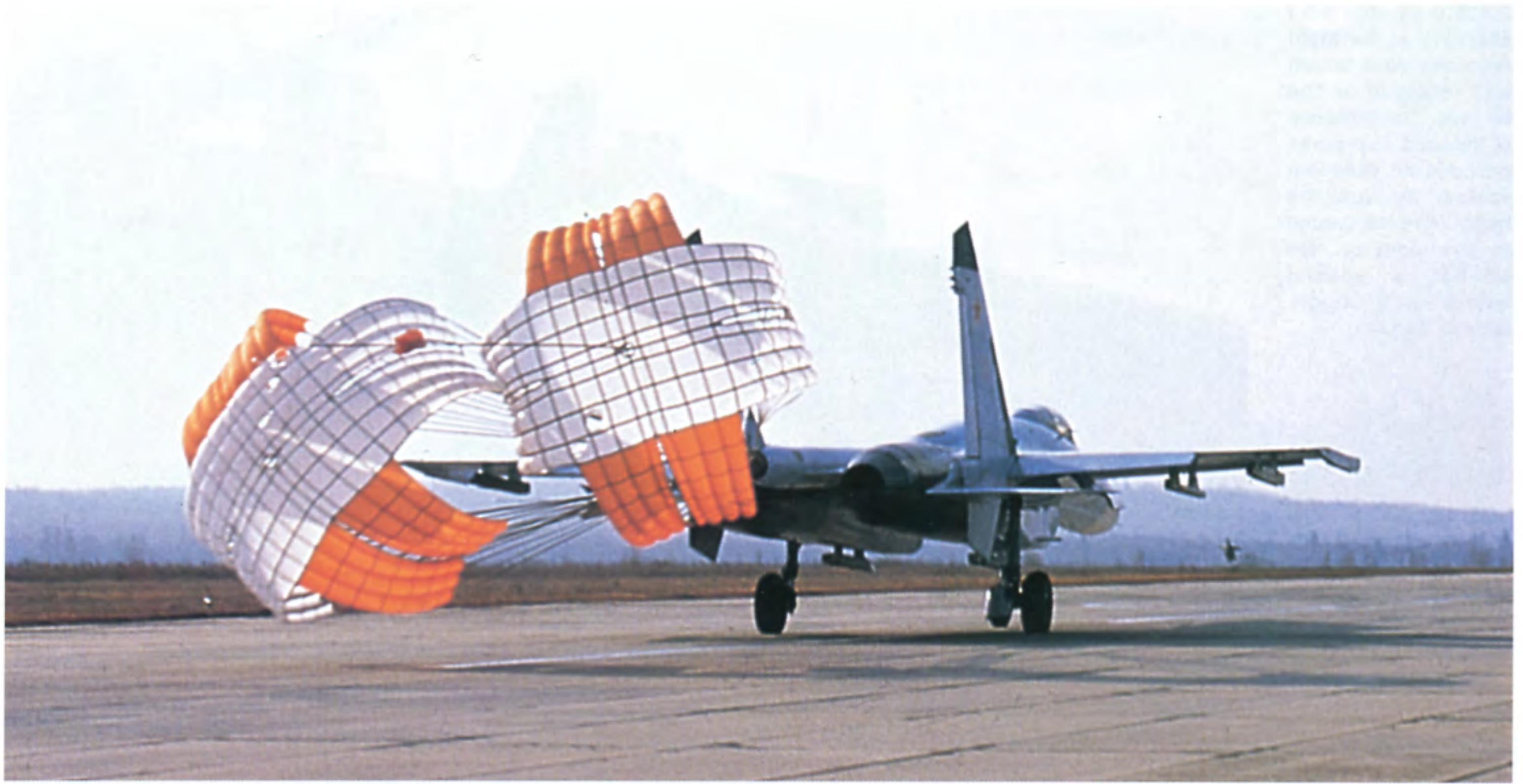
With brake chutes deployed, the Su-27 completes its landing run. It takes about 600m for the aircraft to come to full stop. Note the design of the parachutes. (Leonid Yakutin)
