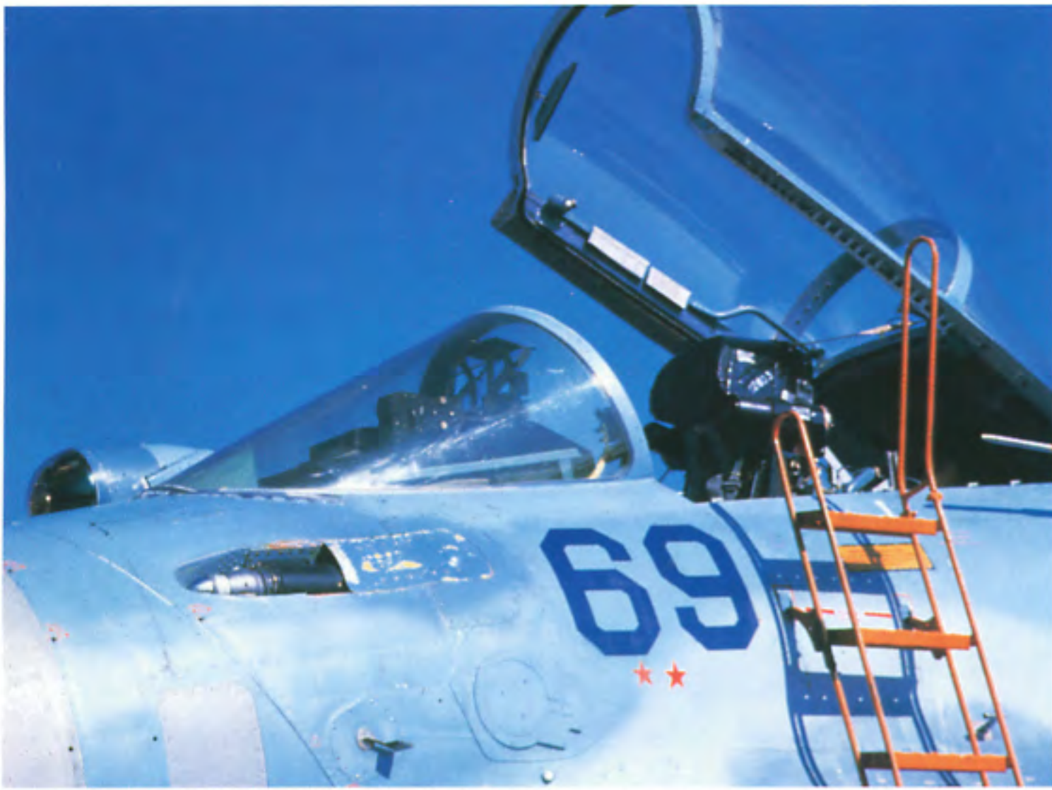
To improve "straight-down" visibility, theIRST ball on Su-27K was offset slightly to the right. The two red stars on the nose of the Su-27K indicate two practice targets destroyed. Note the Head Up Display (HUD) apparatus visible through the windscreen.
