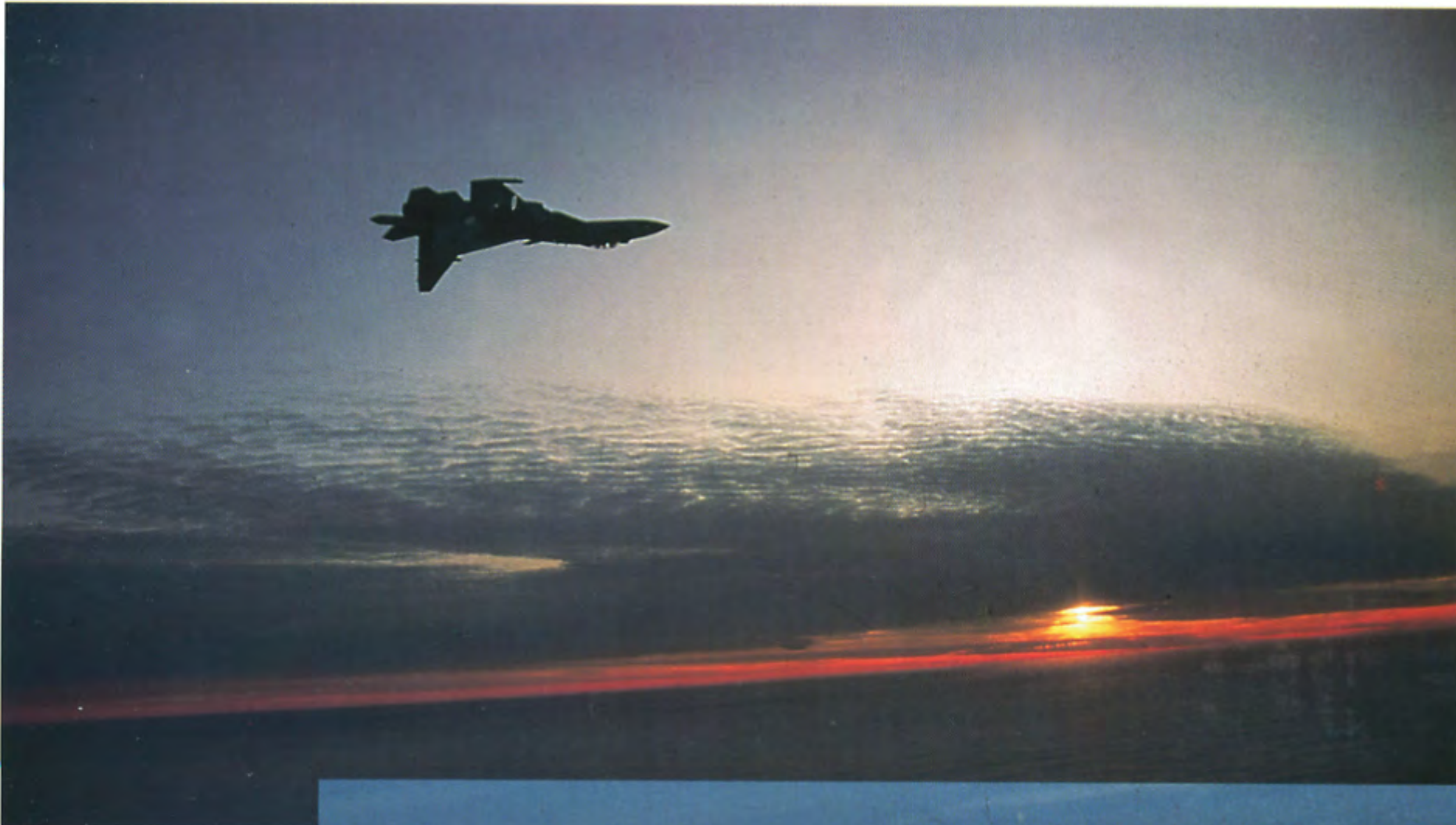
Here a brand new Su-35 overflies the Russian Far East. Its canards are just visible behind the cockpit. These aerodynamic forewings give the aircraft short-field capability and agility.
