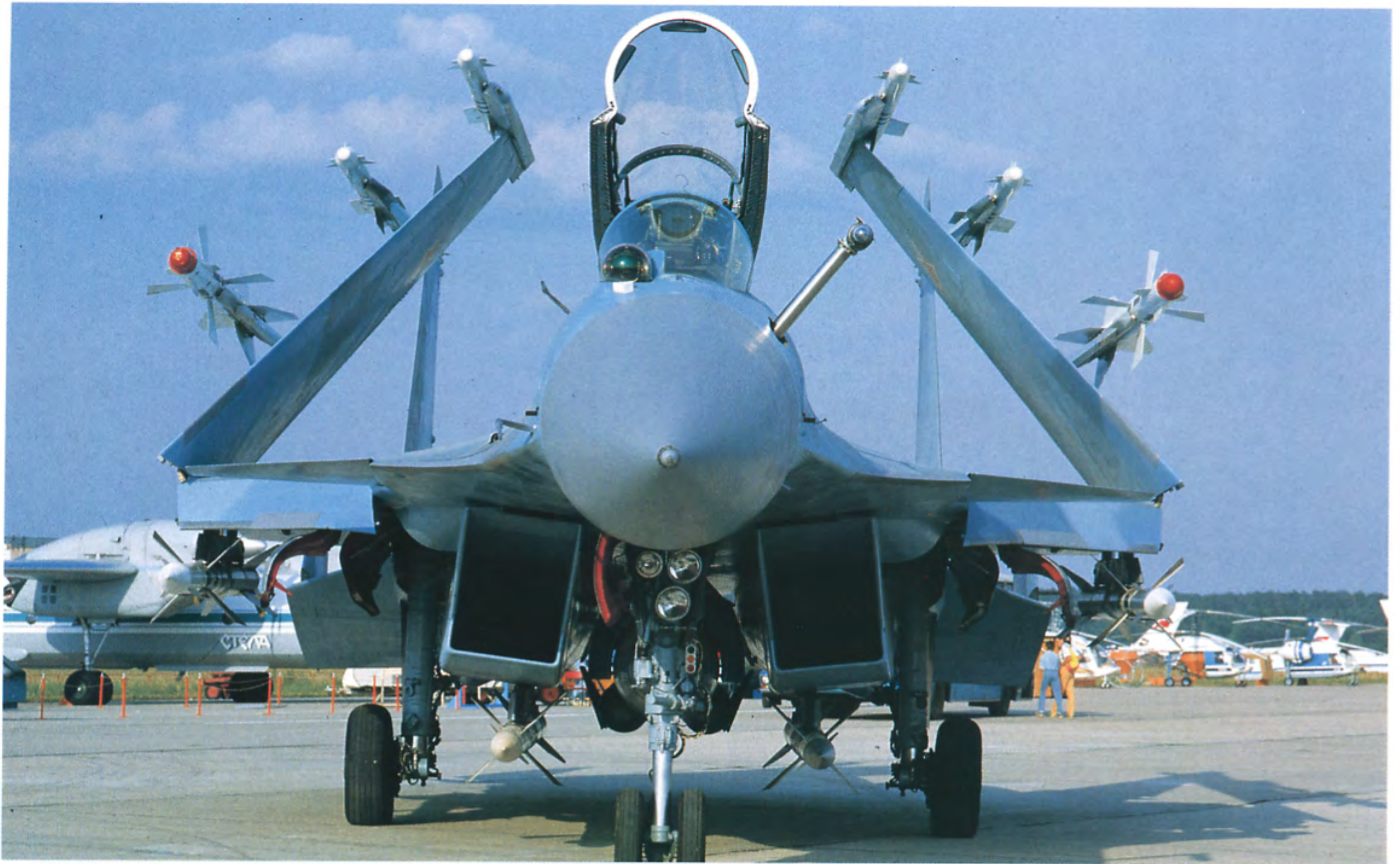
Twelve hard points on the Su-27K allow it to carry a wide range of weaponry from small dogfight AAMs to huge antiradiation and antiship missiles. Notice how the wings of the navalized Flanker are hinged for efficient storage. The in-flight refueling probe protruding from the nose is retractable.
