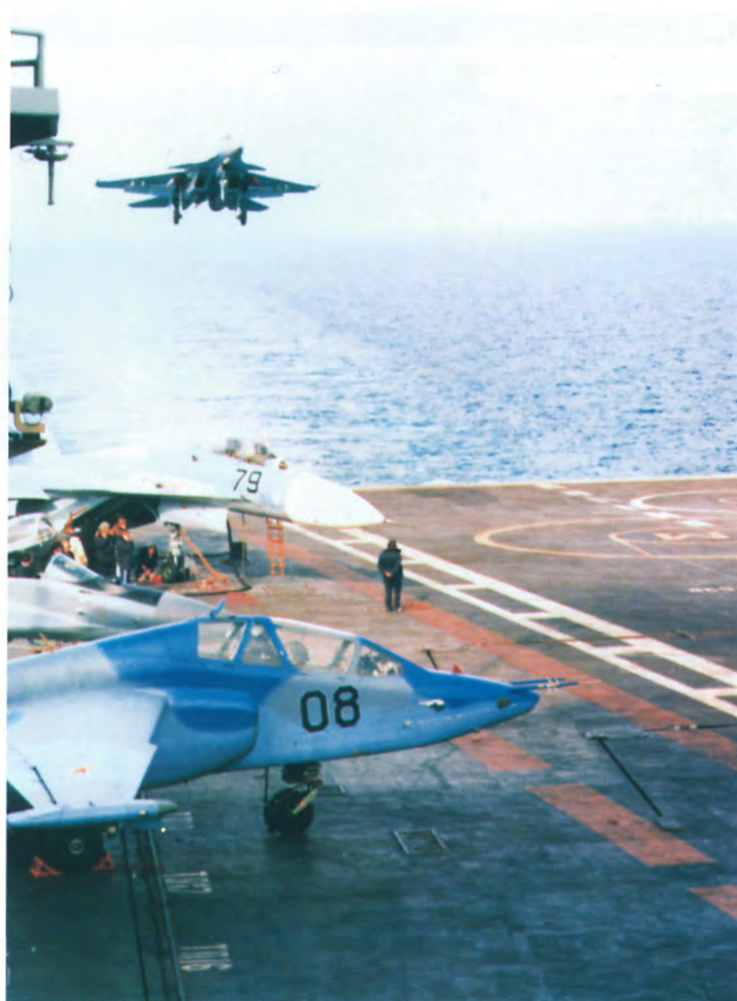
With the pilot strapped in and the retractable chocks raised, this Su-27K is waiting for take-off clearance before it begins its mission over the Black Sea. The aircraft is armed with AA-11 Archers for self-defence and medium range air-to-air AA-10 Alamos. The dielectric panels and radome are painted differently on this navalized Flanker.
