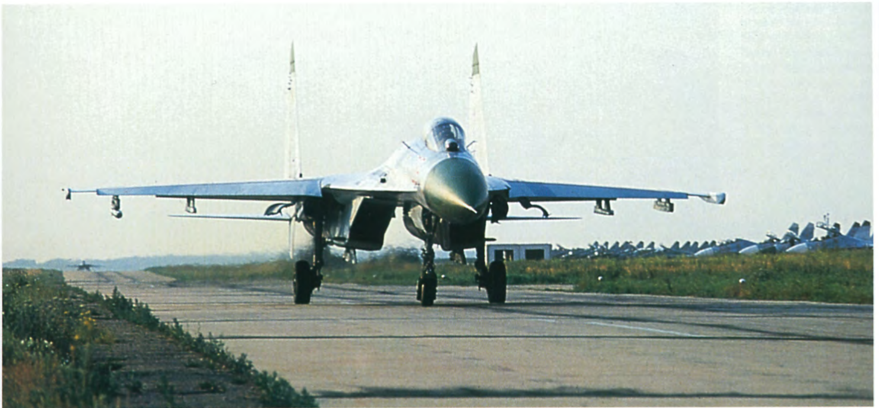
Returned from flight the aircraft still carries a single AA-11 Archer IR homing missile on the portside wingtip only. This photo provides a good view of the box-shaped air intakes. Note how the leading edge slats are deployed.
