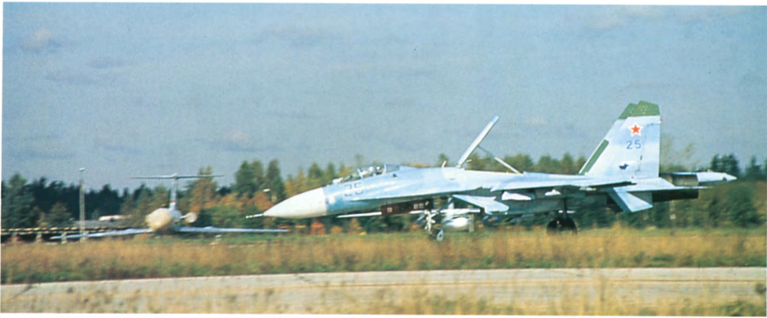
A Flanker with its dorsal speed brake fully extended returns home. Note the unique profile attained when the dorsal brake is used. The paint scheme of this Su-27 is typical of Flankers that are in-service.
