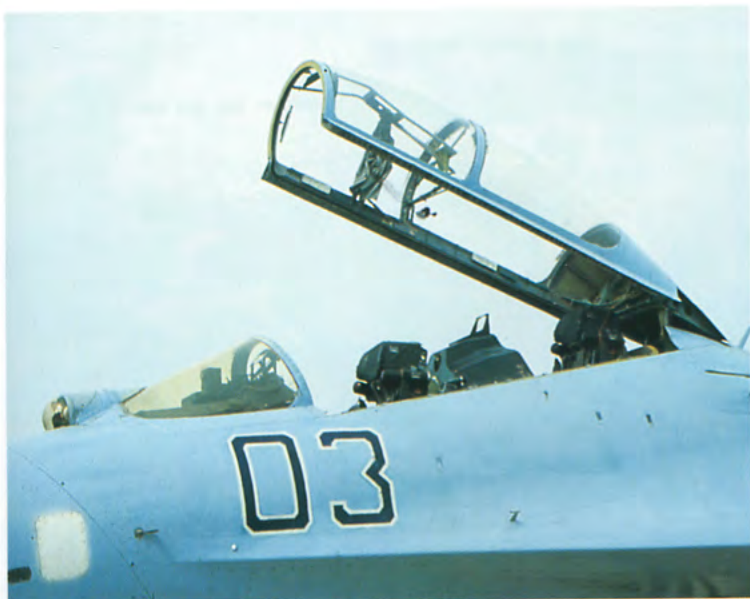
Forward and aft cockpits are covered by a one-piece canopy. It has rear view mirrors for both pilots attached to it. The canopy is mostly free of obstructions and allows excellent viewing. (Yefim Gordon)
