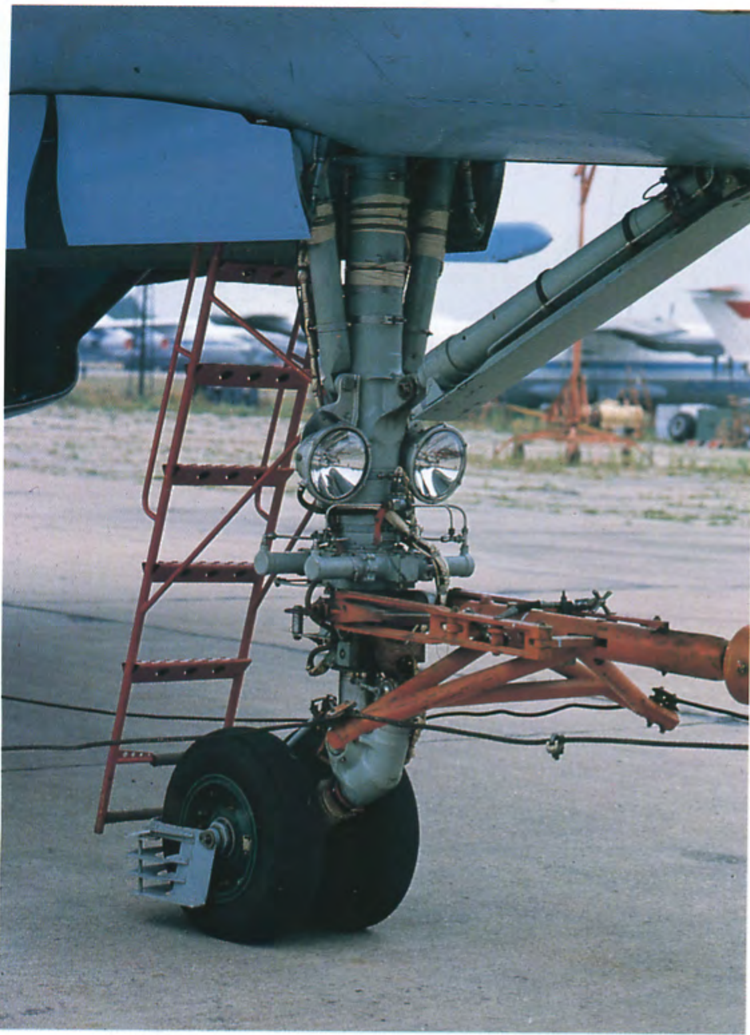
The Su-27IB's crew ingress via the nosewheel bay is a distinct feature of the aircraft. It was a pure novelty for Sukhoi Design Bureau. Unknown design considerations have led to deviation from the conventional layout of the side-by-side cockpit used earlier on the Su-24 Fencer.
