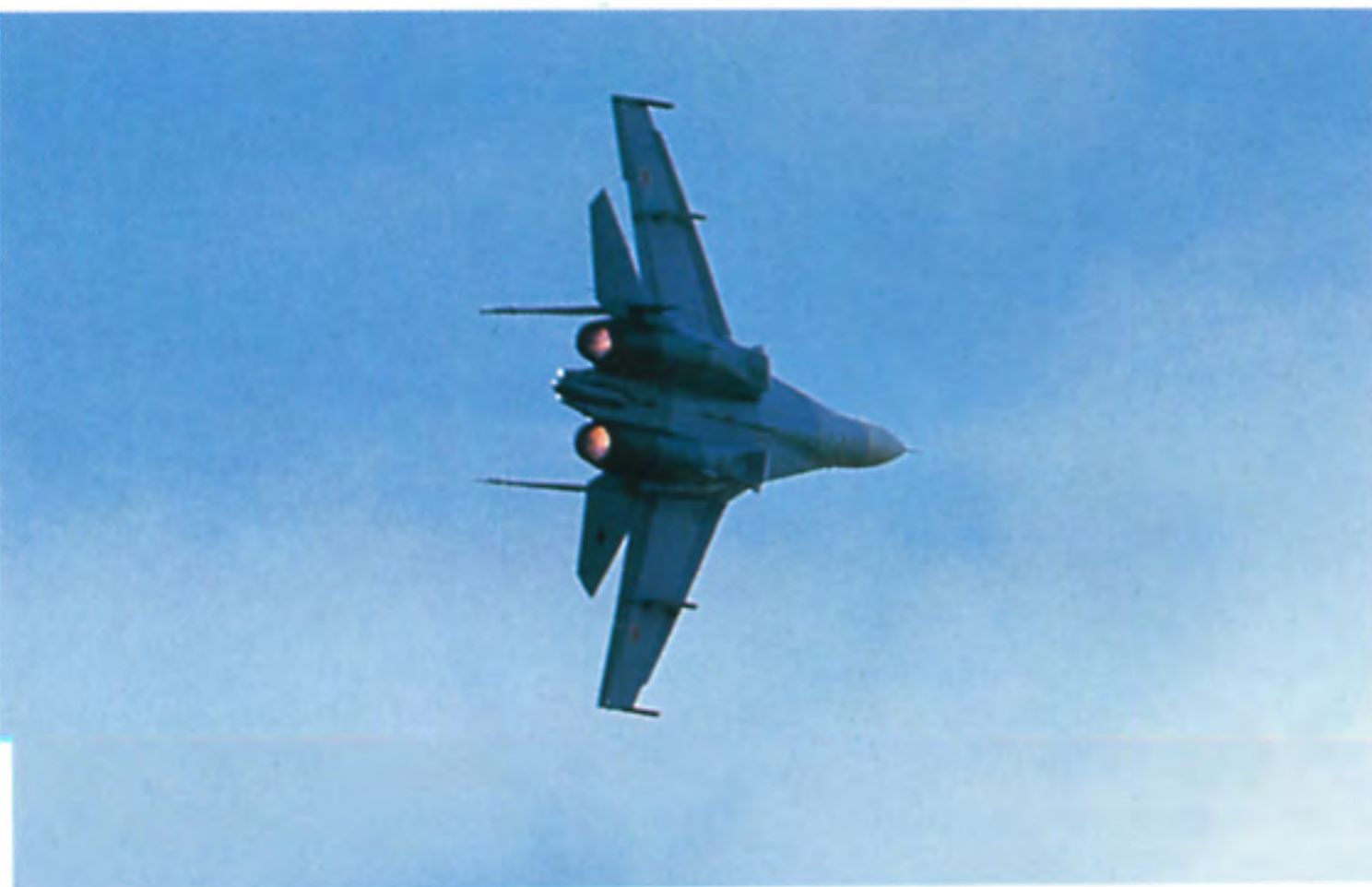
Rear in-flight view of the Su-27 flying with afterburner lit. Visible convergent/divergent nozzles are the radial fuel sprays in the A/B flame stabilizers. The aircraft is powered by two Lyulka AL-31F engines. (Sergey Pashkovsky)
