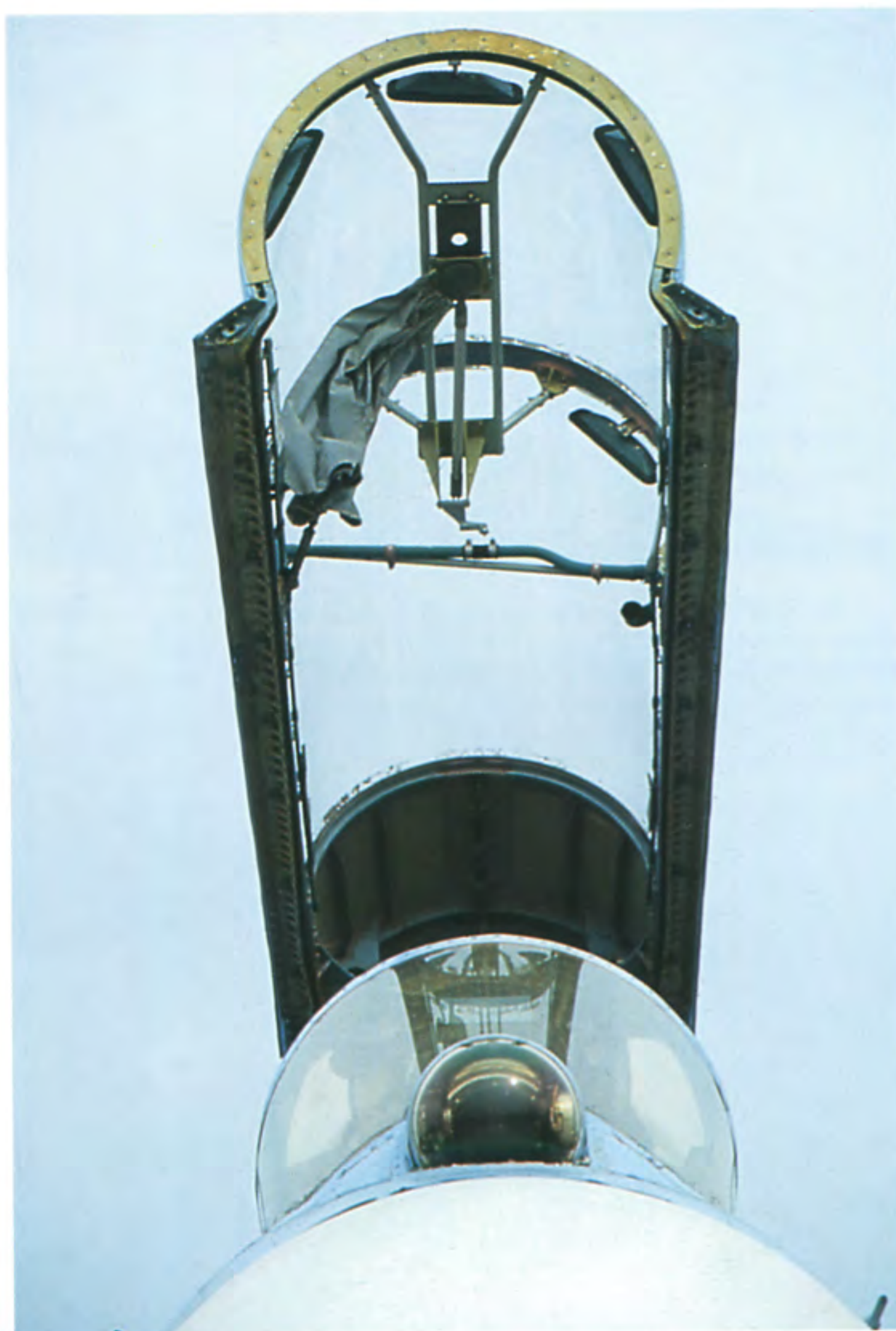
The canopy of the two seat combat trainer is fitted with curtain used to teach cadets IFR mission. In this picture it can be seen pushed to the side near the front portion of the open canopy. The structure of the canopy's interior is displayed well here. (Yefim Gordon)
