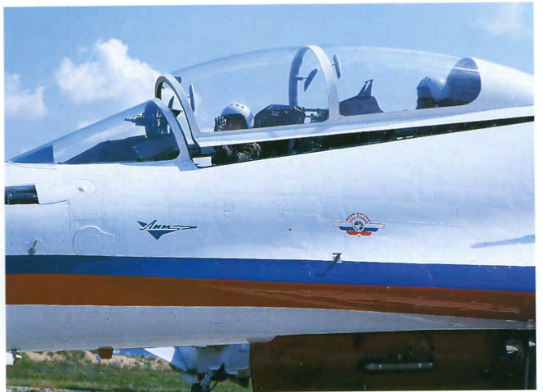
The Su-27PU's cockpit sits high off the ground so access to it is via ladders with attachment hooks above top rung. These ladders are visible on the opposite side of the cockpit. The red undersides of the Flanker is a bright contrast to the traditional camouflage.
