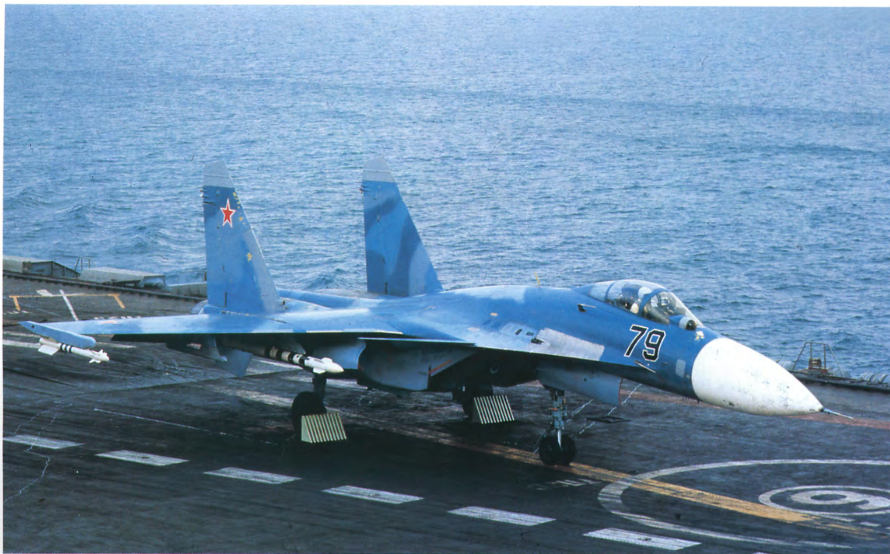
With the pilot strapped in and the retractable chocks raised, this Su-27K is waiting for take-off clearance before it begins its mission over the Black Sea. The aircraft is armed with AA-11 Archers for self-defence and medium range air-to-air AA-10 Alamos. The dielectric panels and radome are painted differently on this navalized Flanker.
