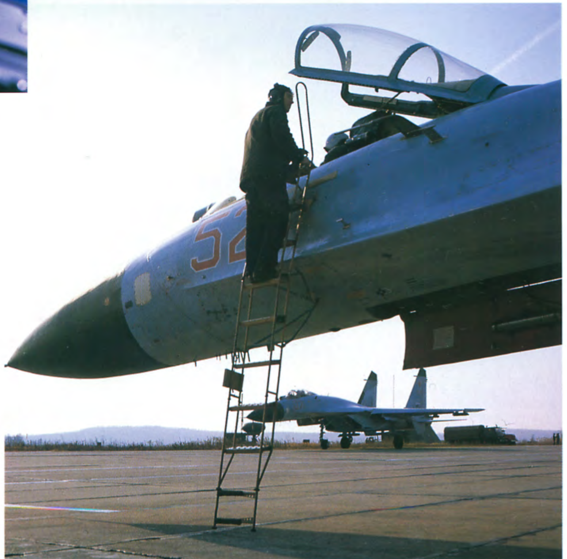
A brown-suited ground crewman stands atop a ladder to help the pilot perform pre-flight functions. In operational units, the technician usually helps the pilot to connect the intercom cable, oxygen mask and G-suit to the cockpit connectors. The ladder was designed for the specific use of pilot and crew. (Leonid Yakutin)
