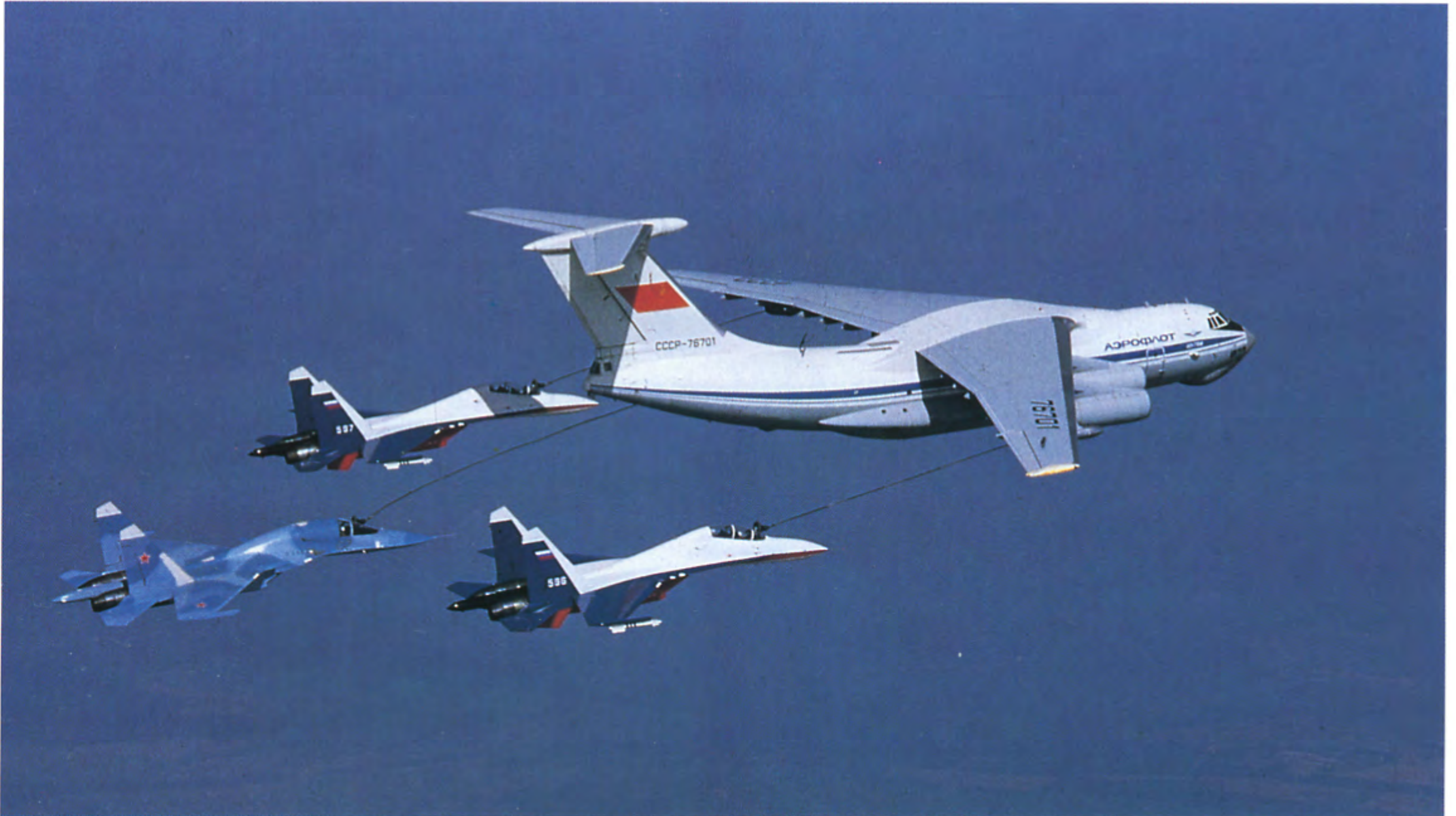
Mixed in-flight refueling of three Sukhois - a pair of Su-27PUs and single Su-27IB from a Ilyushin IL-78 Midas tanker. The size of the Midas tanker is impressive. Note the red section on the tail fin. It looks like it might be the old Soviet flag.
