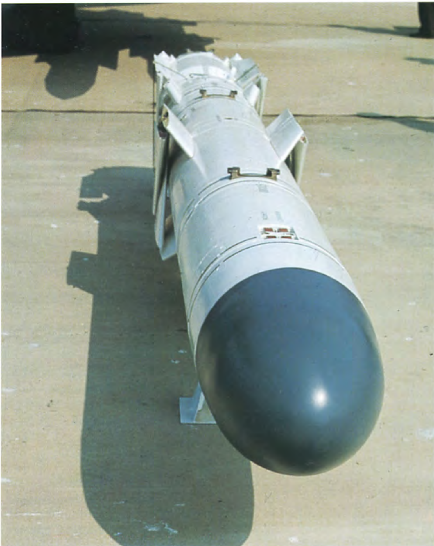
The Kh-35 antiship missile is similar to the McDonnell Douglas Harpoon. It is said to use inertial navigation coupled with active radar-homing. The missile has an engagement range of about 130km.
