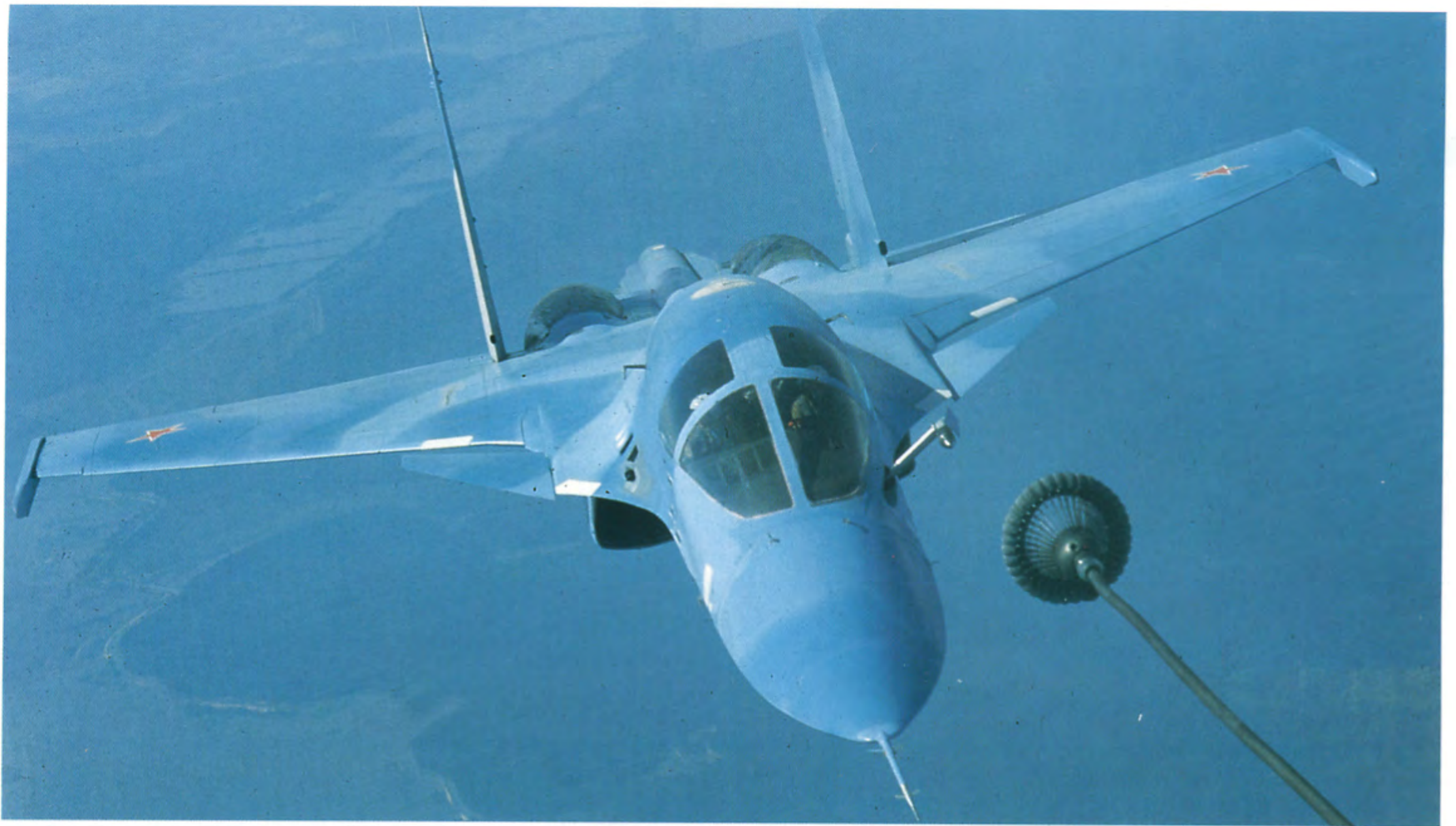
The Su-27IB eases up to the refueling position behind an Ilyushin IL-78 Midas tanker. Note the extended refueling probe. This essential procedure eliminates the need for extra fuel tanks which would limit performance.
