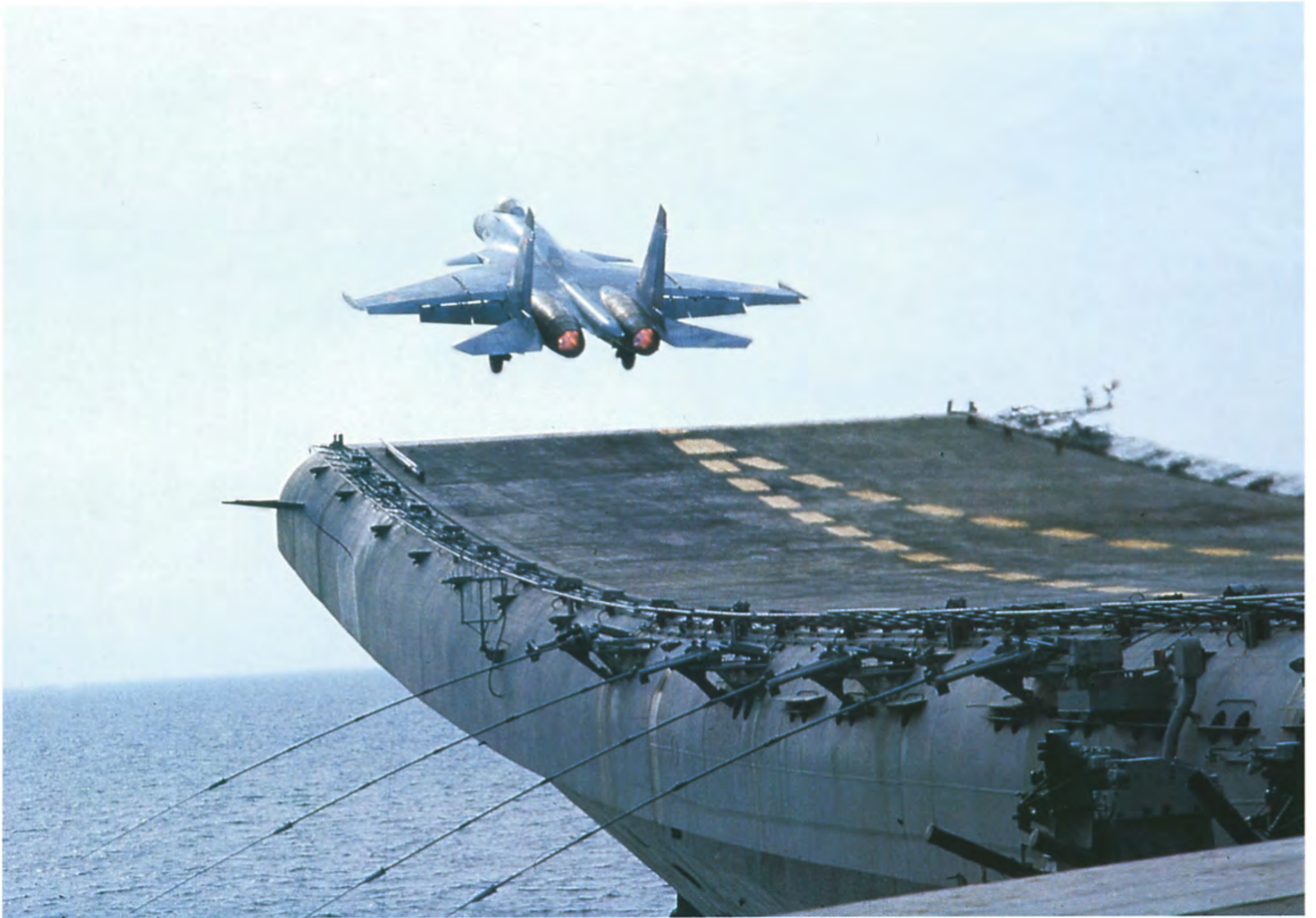
Here a navalized Flanker shoots airborne by means of a main deck's 12 degree ski-jump. The afterburner acceleration gives the aircraft an added boost.
