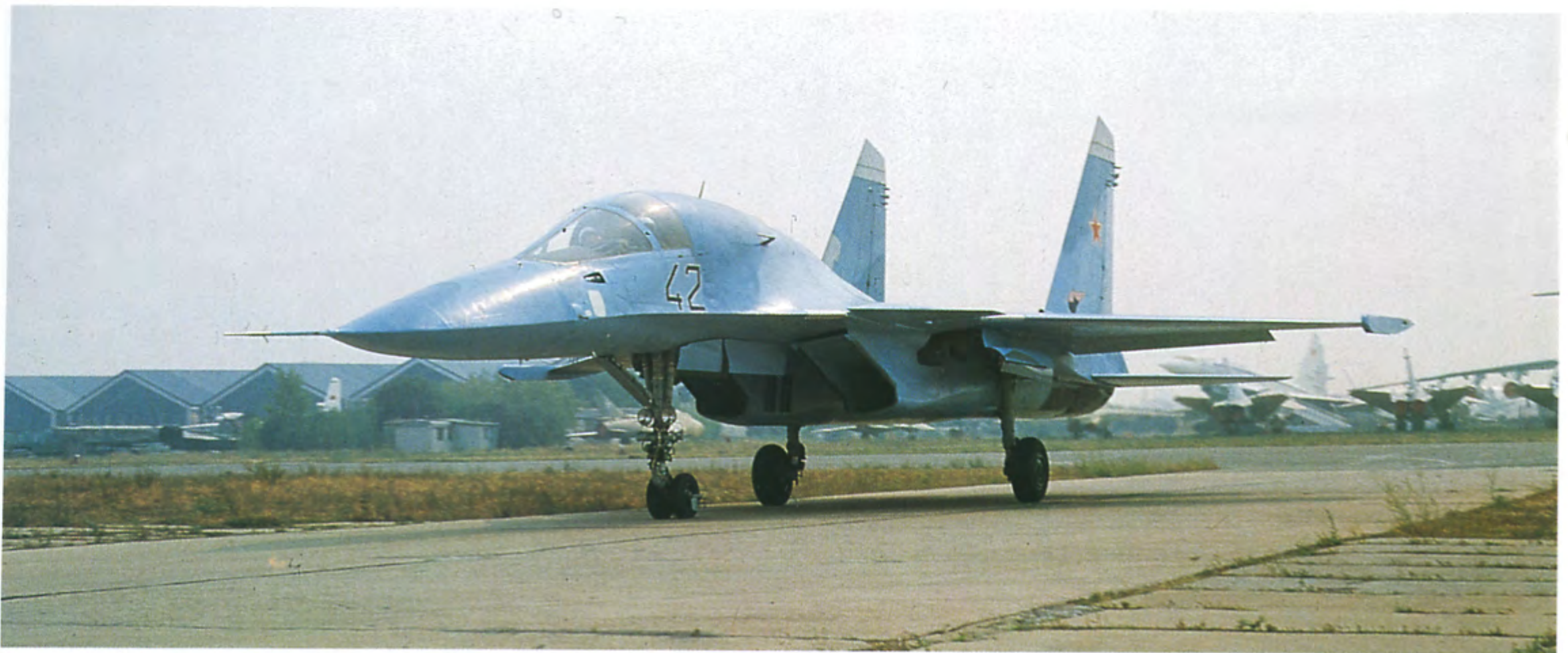
Su-27IB is readily distinguished from other members of the Su-27 family with side-by-side cockpit and the unusual hard-edged front fuselage. The noticeably enlarged dorsal fairing is another new feature. The canards are similar to those used on the navalized Su-27.
