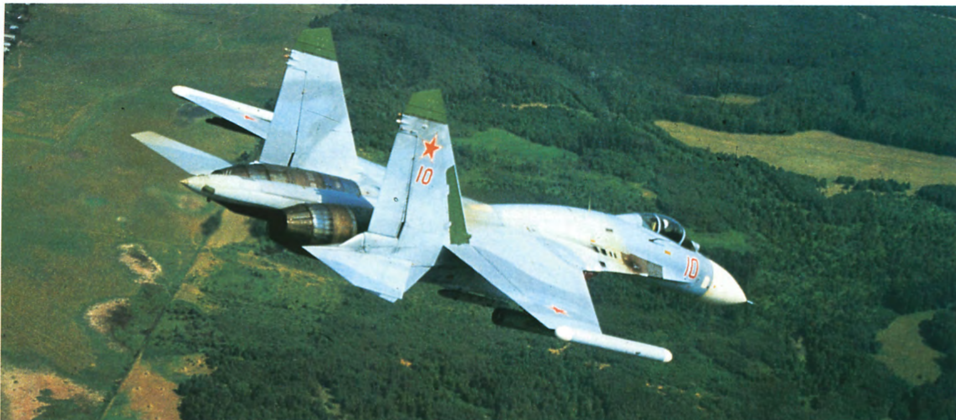
Dirty black residue around the GSh-301 cannon's muzzle reveals gun firing practice took place during this mission. The discoloration will be removed from the blast shield immediately after landing. The blast shield on the Su-27 is made of titanium.
