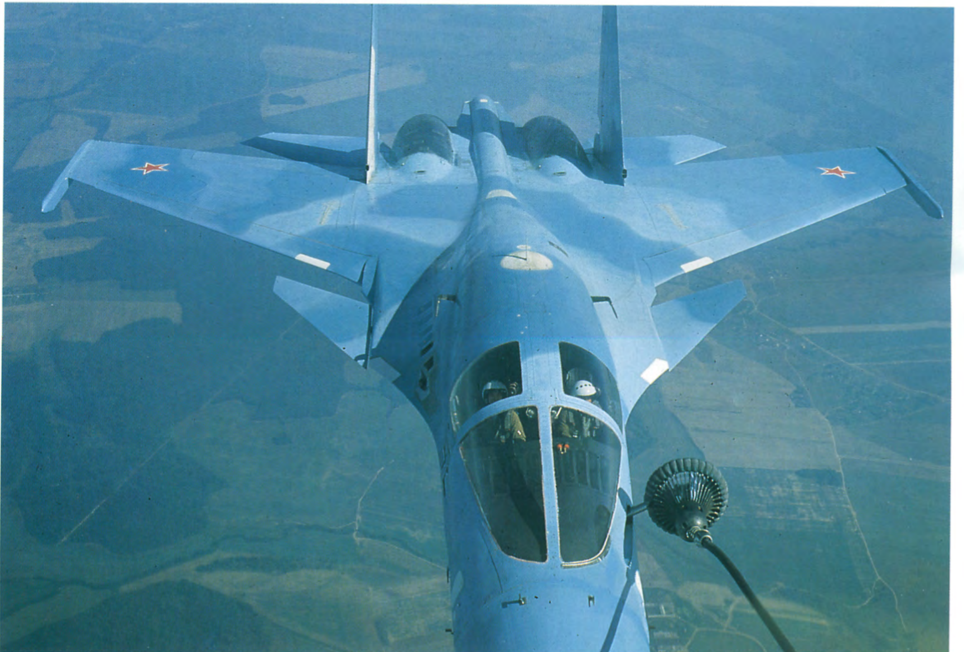
In this photo, the Flanker's refueling probe is hooked to the refueling line of an unseen Ilyushin IL-78 Midas tanker. Note the small canards forward of the main wing. Along with the side-by-side cockpit and hard-line nose, these are the distinctive features of the Su-27IB.
