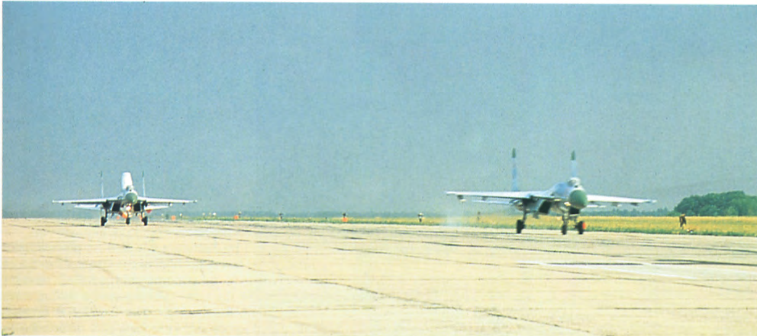
Su-27 landings are frequently made without a drag chute in operational Air Force units. Instead, dorsal airbrakes and wheel brakes are used to moderate extent. Sometimes, the nose is raised to create drag against the underside of the wing.
